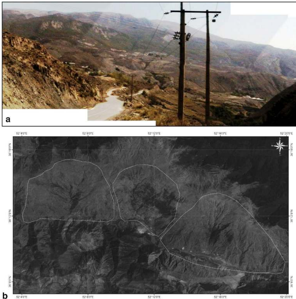
Fig. 5 a Part of Razan landslide complex in the field. b Razan landslide complex divided into three landslides, Doab, Razan, and Ina landslides in Band 7 ETM +
