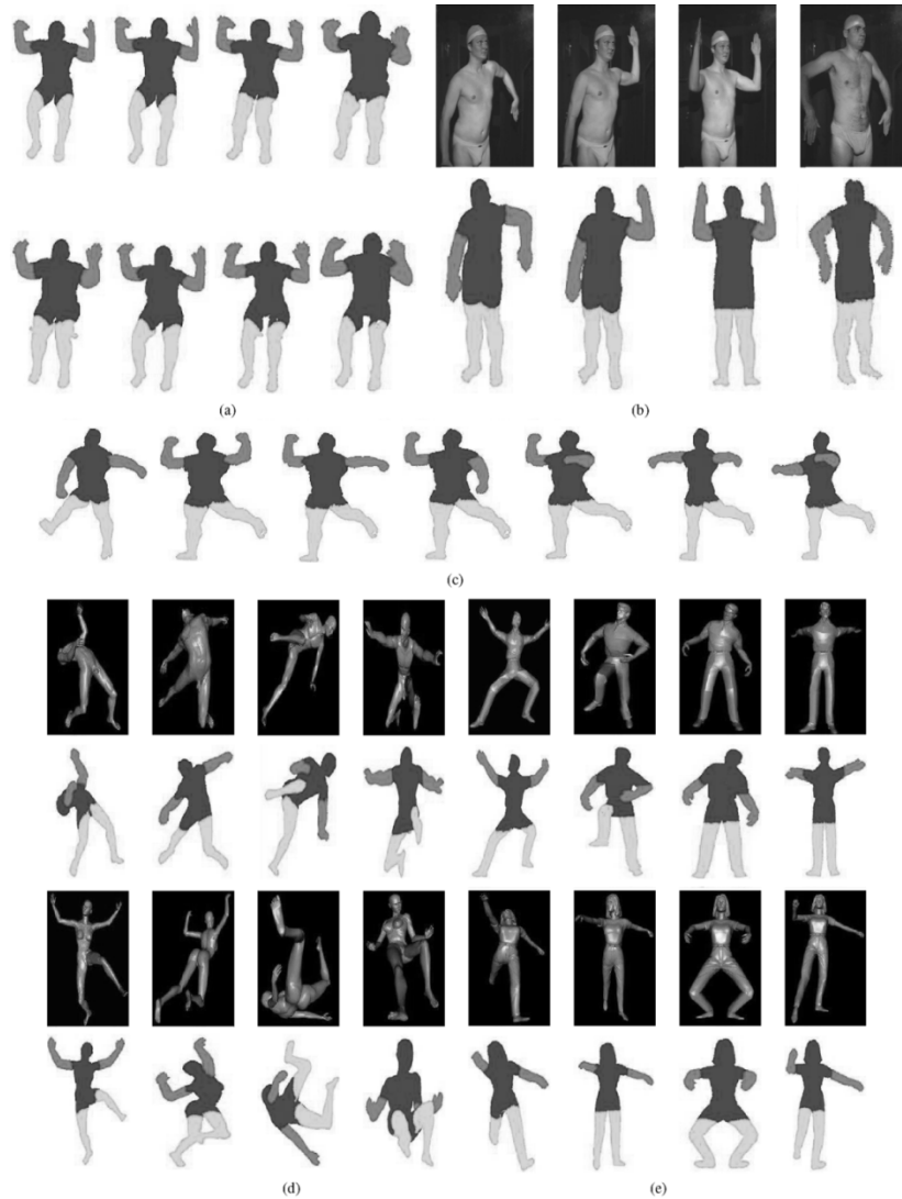
Fig. 8. (a) Segmented real scans corresponding to setting postures acquired with the Cyberware scanner. (b) Segmented Wick & Wilson scans related to nonstandard postures. (c) Segmentation results of an animated Cyberware scan. (d) and (e) Segmentation results of simulated scans corresponding respectively to scans of naked and dressed characters.
