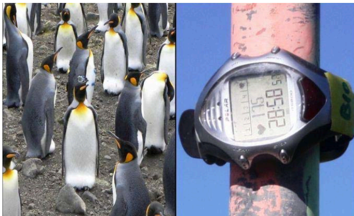
Fig 3. Heart rate monitoring of breeding penguins in their natural environment. The transmitter of the HR-logger is taped to the feathers in a mid-dorsal position to prevent hindering movements from the bird and to be out of reach of the animal. The receptor is attached to a plastic flipper-band, loosely secured to the animal's flipper (left panel), or attached to a metal pole placed close to the incubating/brooding bird (right panel). When visible, the digital display allows monitoring HR (175 bpm in this case) from a distance, using binoculars. Taken from [91] .
