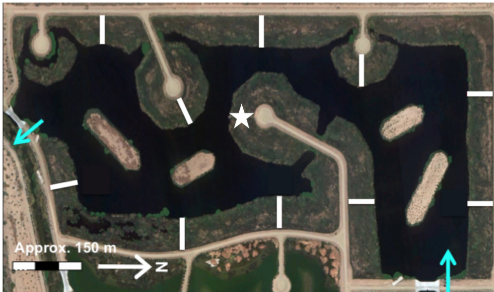
Figure 14: Aerial image of the 42-ha Tres Rios constructed treatment wetland. White lines are the locations of the 10 marsh transects (each 50–60 m long), and blue arrows show the water inflow and outflow points. The star indicates where the July 2015 controlled-flow dye study was conducted
