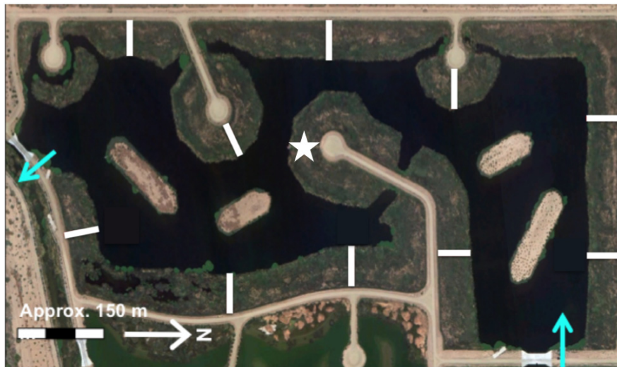
Fig. 1. Aerial image of the 42-ha Tres Rios constructed treatment wetland. White lines are the locations of the 10 marsh transects (each 50–60 m long), and blue arrows show the water inflow and outflow points. The star indicates where the July 2015 controlled-flow dye study was conducted.
