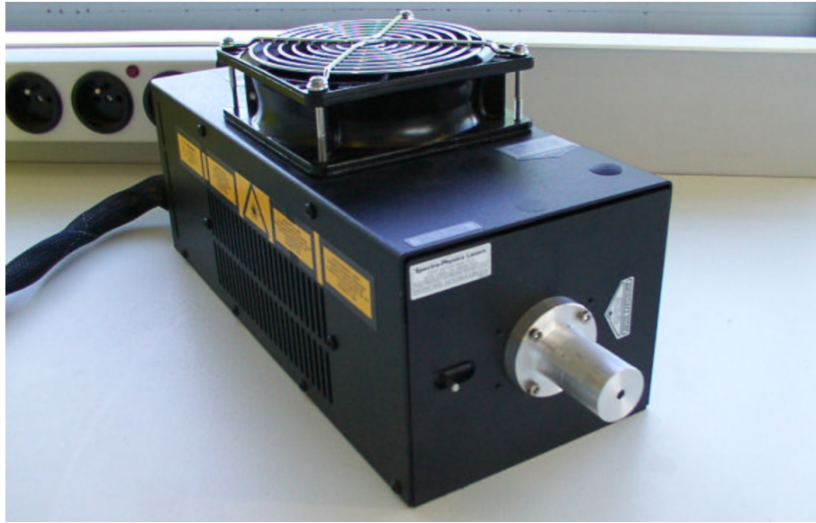
Figure 5.17: Mechanical integration of the diffractive beam shaper onto the laser head package.
