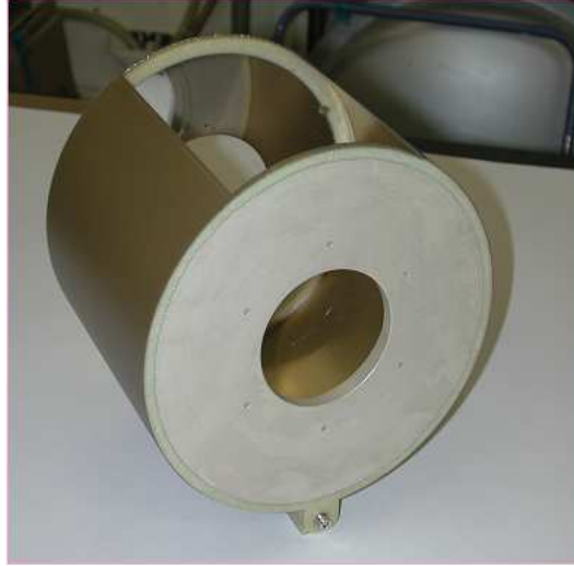
Figure 4.9: The cylindrical cage wall of the first prototype made of gold/copper coated fibreglass with the 60° degrees arc covered with a tungsten wire grid. The ring electrode at the cage exit is made of stesalite covered with conductive silver paint except for a 5 mm thick outer ring, visible in the picture, for the electrical insulation between cage and ring electrodes.
