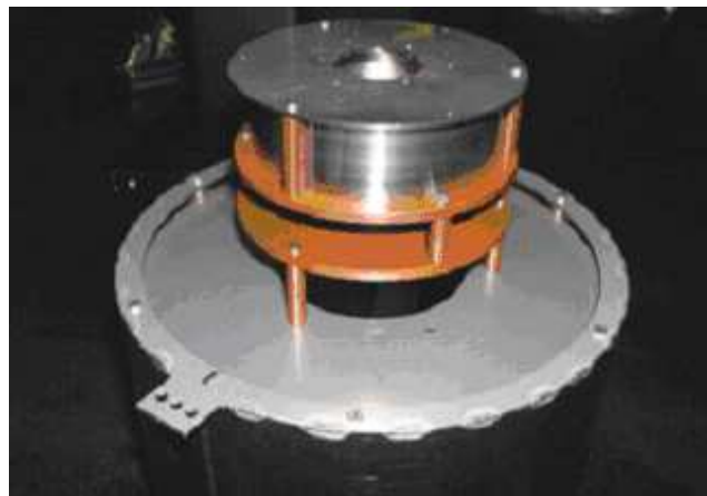
Figure 4.14: Improved focusing system with detail of the cylindrical electrodes on the detector side.
