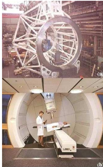
Figure 1.10: The NPCT isocentric rotating gantry: mechanical support (a) and treatment room equipment (b).
