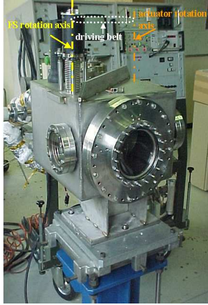
Figure 5.2: Drawing of the FS rotation system (the actuator has been fixed on an aluminium support to have the rotation axis in the position indicated in orange).
