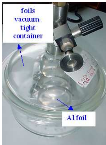
Figure 4.19: The aluminium foils that underwent the full treatment mounted on a stainless steel support, ready to be mounted on the focusing system for the beam tests. The foils are conserved in a primary vacuum container.
