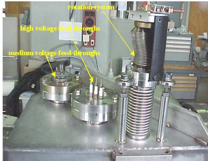
Figure 4.7: SLIM beam monitor vacuum system, detail with the polarization feed-throughs and the rotation system.
