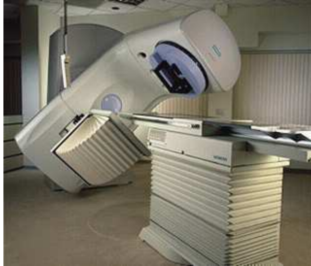
Figure 1.8: Modern linear accelerators for photon and electron treatments rotate around the patient to direct the beam to the target from any direction.
