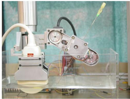
Fig. 3.7: L'Ultrasound-guided Motion-adaptive Instrument [HDH<sup>+</sup>02].
