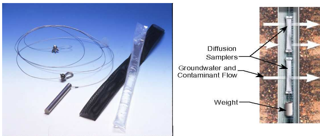
Figure 1-9: Le Passive Diffusion Bag (PDB)
