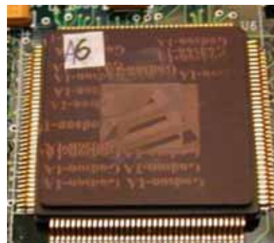
Godson Chip, Godson Chip Industry Alliance The “dragon chip” is a nickname for computer chips recently developed in China as an alternative to US-made Intel and AMD chips.
