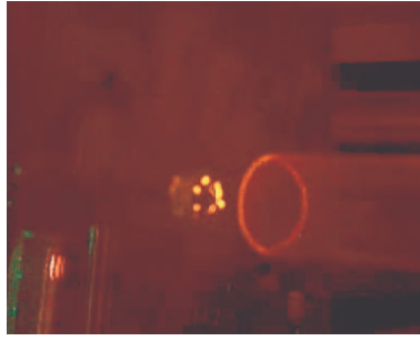
Figure 3.4: Self-focusing of the beam after SHG describing a ring according to a super Gaussian profile beam theory.
