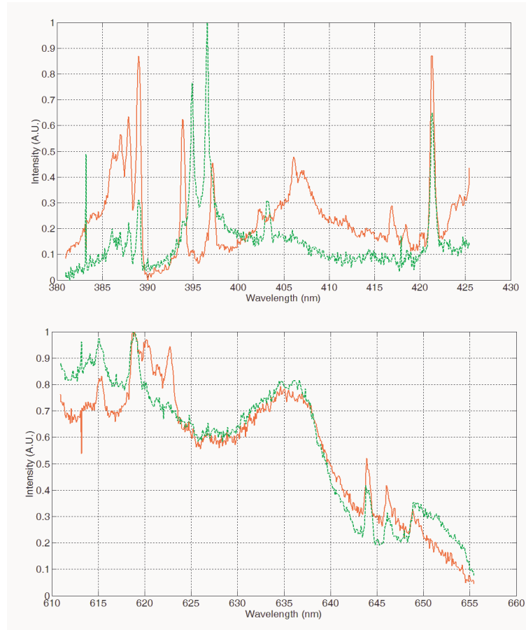
Figure A.2: Top: Dotted lines: Spectra of DNT on Copper obtained by LIBS with filaments, Full lines: Spectra of DNT on Aluminium obtained by LIBS with filaments, Bottom: Dotted lines: Spectra of ammonium perchlorate on Copper obtained by LIBS with filaments, Full lines: Spectra of ammonium perchlorate on Aluminium obtained by LIBS with filaments,
