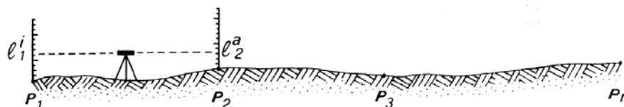
Figure 2.5: Schematic procedure used for geometric leveling: measurements of benchmarks ( P_1 and P_n ) along a levelling line (modified after Muller, 1986)
