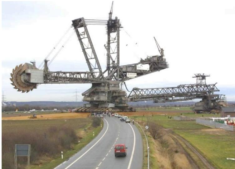
**Figure 1.** The giant mining excavator, Bagger 288, built by Krupp<sup>[2]</sup>
