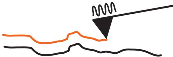
**Figure II.7:** Schematic representation intermittent imaging mode.
