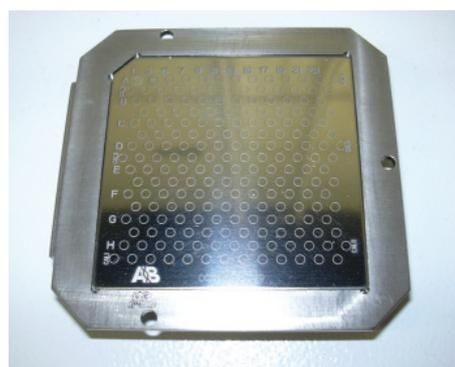
**Figure I.5:** Example of a 192 sample wells MALDI-plate
