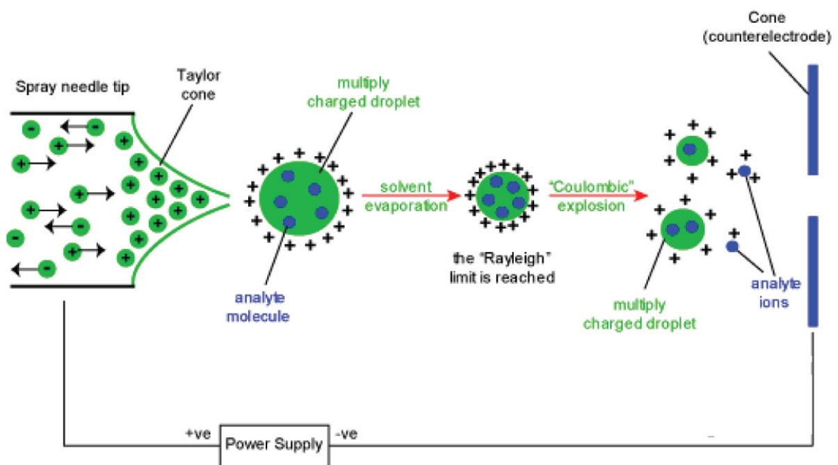
**Figure I.3:** A schematic representation of the mechanism of ion formation (Fig. from: <http://www.bris.ac.uk/nerclsmf/techniques/hplcms.html>).
