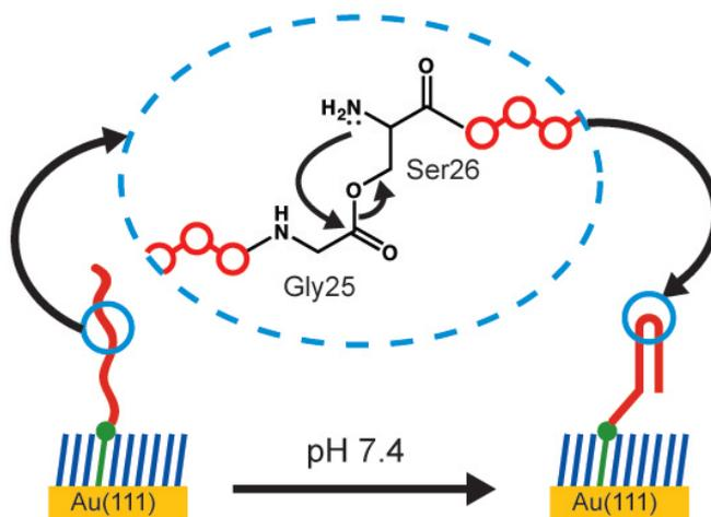
**Figure 3:** O-N intramolecular migration reaction on the functionalized gold surface.
