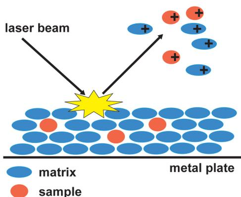
**Figure I.4:** Schematic representation of MALDI process
