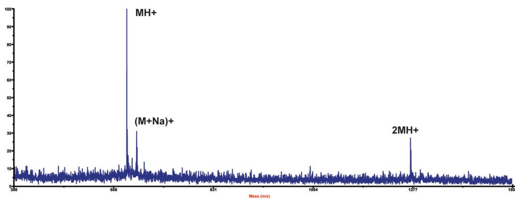
**Figure 5:** MALDI-MS spectrum of the N-Lys-(penta-PEGylated) alkanethiol; Theoretical mass =  $MH+ 637$  Da.
