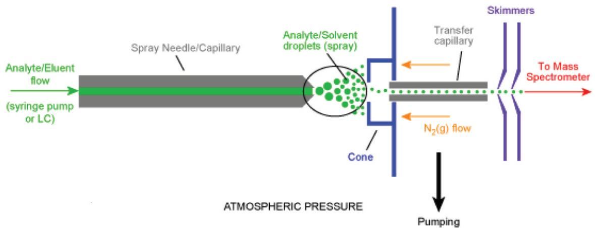
**Figure I.2:** Schematic representation of the electrospray source interface (Fig. from: <http://www.bris.ac.uk/nerclsmf/techniques/hplcms.html>).
