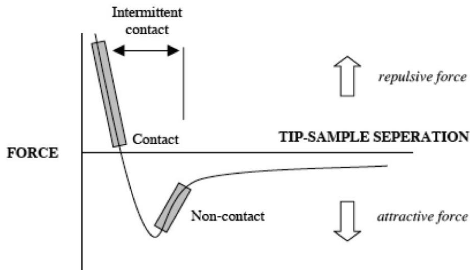
**Figure II.4:** Variation of the forces with tip-sample separation during the three main AFM imaging modes
