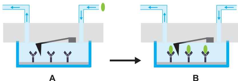
**Figure II.16:** Schematic representation of an experimental set-up to perform in-situ AFM studies under liquid conditions; liquid can be injected into or removed from the liquid cell without perturbation to the system.
