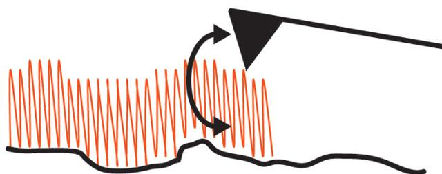
**Figure II.6:** Schematic representation of intermittent imaging mode.
