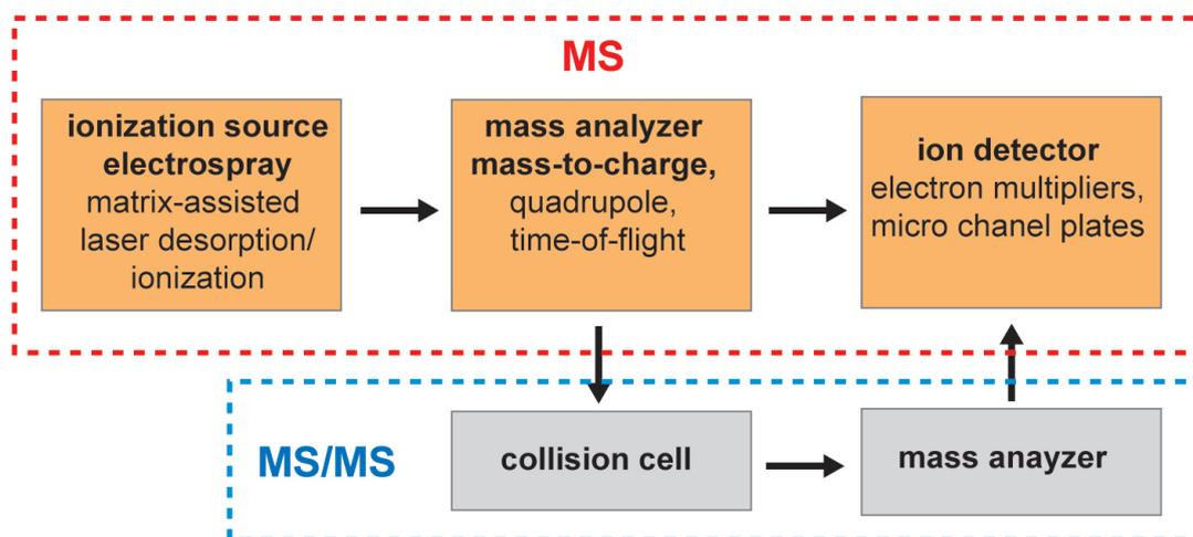
**Figure I.1:** Schematic representation of a mass spectrometer
