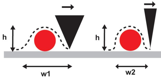
**Figure II.3:** Schematic representation of a sample imaging by two tips having different cone angle. A first image is obtained and the height ( $h$ ) and the width ( $w_1$ ) of the sample is measured; the same sample is then image with sharper tip: resolution improved ( $w_2$ ) but height measurements stay uniform ( $h$ )
