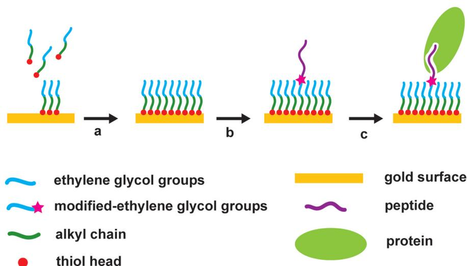
**Figure I.9:** Self-assembled monolayer formation for SAMDI analysis in protein interaction studies. (a) formation of the SAM with ethylene-glycol-groups-terminated alkanethiols and modified ethylene-glycol-groups terminated alkanethiols; (b) peptide immobilization; (c) the surface is ready for protein interaction studies
