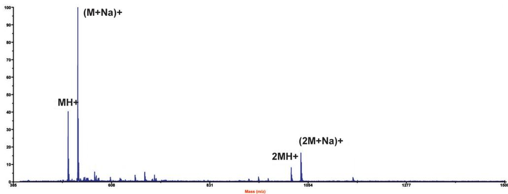
**Figure 4:** MALDI-MS spectrum of the penta-PEGylated alkanethiol; Theoretical mass =  $MH+ 509$  Da
