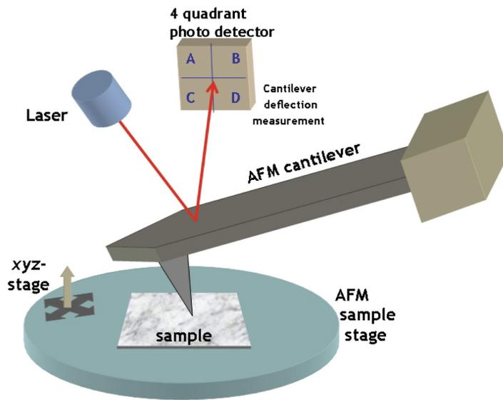
**Figure II.1:** Schematic representation of the atomic force microscope (Image from the Open source Handbook of Nanoscience and Nanotechnology).
