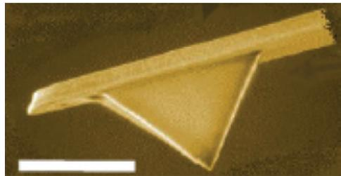
**Figure II.2:** AFM tip, bare scale at  $3\mu\text{m}$
