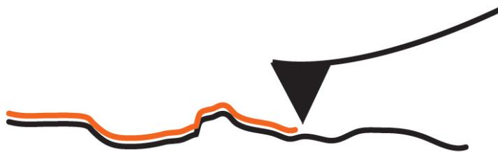
**Figure II.5:** Schematic representation of contact imaging mode.
