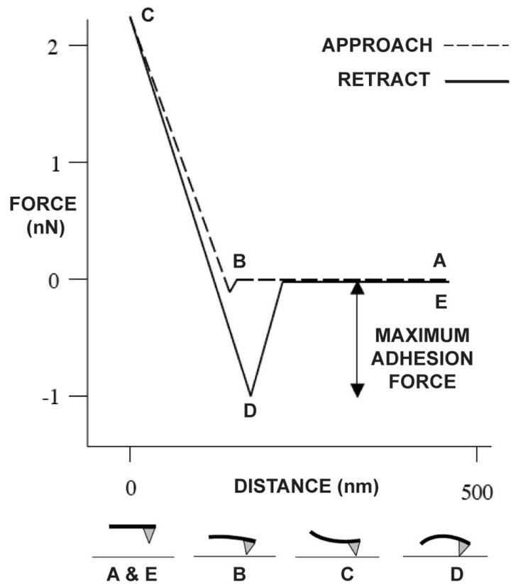
**Figure II.8:** Scheme of a typical force-distance curve observed with the AFM. (A) Tip approaches sample surface, (B) jump to contact due to long range attractive forces, (C) point of maximum load, which is set by the user, (D) disengagement (or pull-off) as tip is retracted from surface and (E) tip returns back to its starting position out of the range of any forces.
