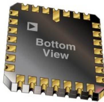
Figure 3.13: Ceramic Leadless Chip Carrier (CLCC) with 28 pins.
