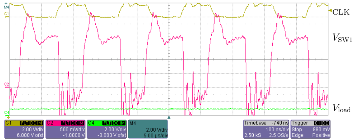
Figure 6.12: Oscilloscope of the IPC2 in buck mode ( V_{\text{batt}} = 1.7\text{ V} , V_{\text{load}} = 1.0\text{ V} , f_{\text{osc}} = 5\text{ MHz} ). The interferences are due to the long signal tracks on the test PCB.
