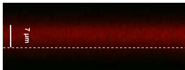
Figure 1. Confocal microscope section (x,z) image of (\text{PLL}/\text{HA})_{30}/\text{PLL}/\text{AP}^{\text{Rho}}/(\text{PLL}/\text{HA})_2 multilayer film deposited on a silicone sheet. The dotted line indicates the interface between the silicone sheet and the multilayer film.
