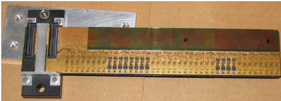
Figure 7.1: A prototype PIXEL ladder design fabricated on a copper conductor cable and populated with nine full-reticule size MIMOSA V sensors thinned to 50\ \mu\text{m} . Three sensors had all four sectors fully operational. The prototype was constructed at LBL.
