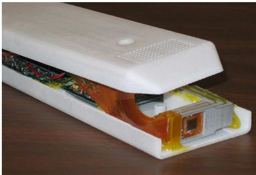
Figure 7.13: Telescope head structure with three MIMOSTAR2 sensors arranged into parallel and coaxial planes.
