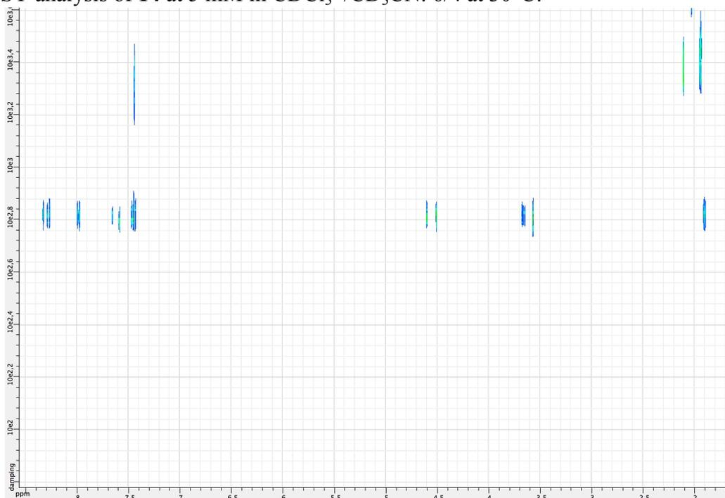
The measured diffusion coefficient ( $D=6.50 \cdot 10^{-10} \text{ m}^2\text{s}^{-1}$ ) gave a hydrodynamic radius of 7.14 Å. When using an ellipsoid model, the following dimension could be found: 5 x 37 Å, which fit well with a model of the ligand.
