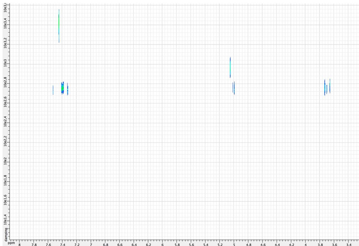
The measured diffusion coefficient ( $D=5.7010^{-10} \text{ m}^2\text{s}^{-1}$ ) gave a hydrodynamic radius of 8.1 Å.
