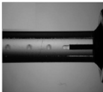
Figure 19. Generation of droplets containing cells using a breakup technique , picture from (Sakai et al., 2005).
