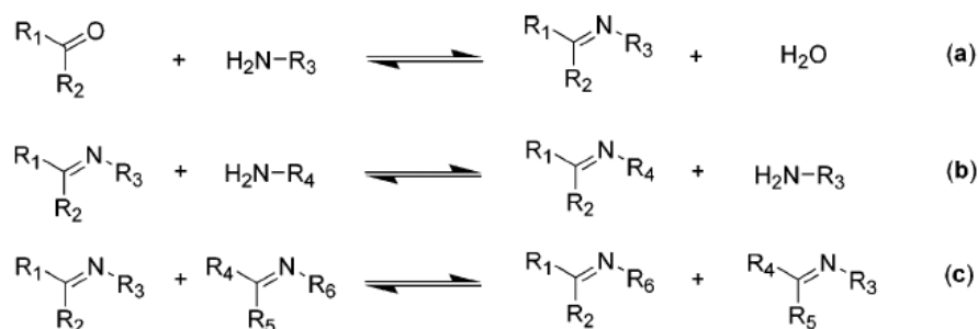
Figure 2-3. Types of Amine Exchange Processes Involving the Imine Bond: (a) Condensation and Hydrolysis; (b) Transimination; (c) Imine Metathesis. [2,8]
