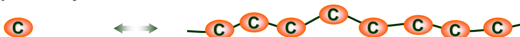
Figure 1-31. Schematic cartoons of dynamers. They may be of the supramolecular type involving polyassociation with interactional recognition or of the reversible covalent type formed by polymerization/polycondensation with functional recognition between the connecting subunits.
