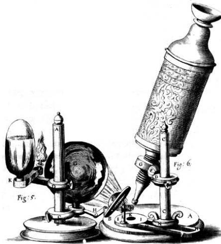
Figure 1.2: Drawing of an optical microscope by Hooke in his book *Micrographia* from 1665 [11].
