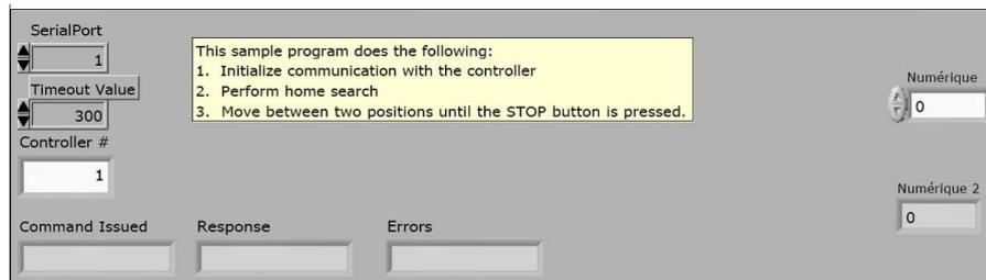
Figure C.5: Control panel of the subroutine program dedicated to the control of the filter wheel.
