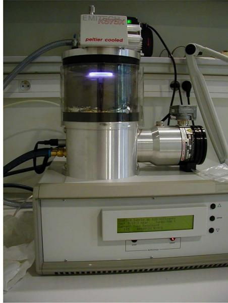
Figure 4.1: Emitech K575x Turbo Sputter Coater during deposition.
