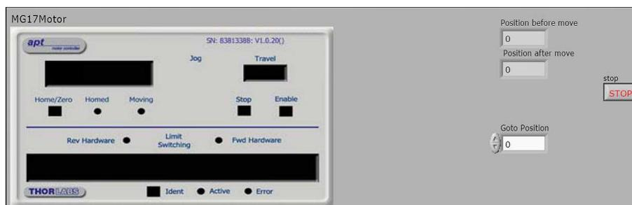
Figure C.7: Control panel of the subroutine program dedicated to the control of the rotation motor unit (Thorlabs T-cube TDC001).
