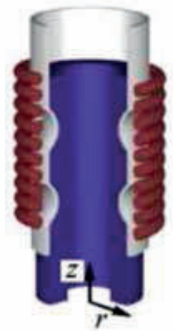
Figure III-21: A schematic view of electromagnetic tube compression process.
