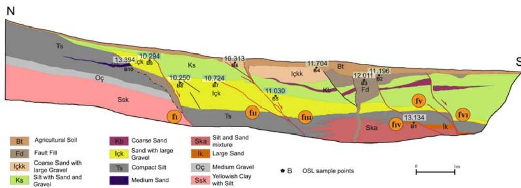
Figure 4.7 Log of Argavlı trench (eastern wall). Main faults are marked as “f<sub>I</sub>” – “f<sub>VI</sub>” (Altunel *et al.*, 2009).
