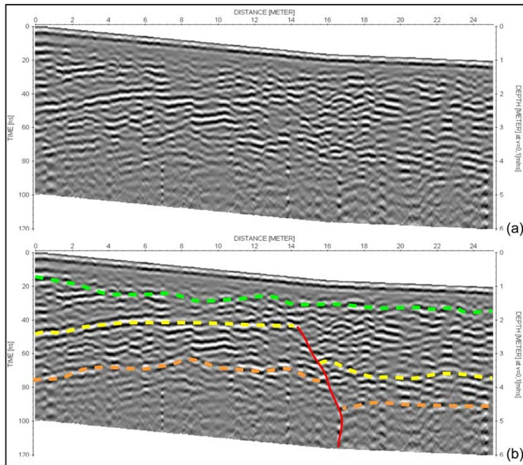
Figure 4.32: (a) Processed data of "GPR\_profile\_3" GPR profile. (b) Interpretation of "GPR\_profile\_3" GPR profile. Dashed lines represent the layers, thin red line represents possible fault zone.
