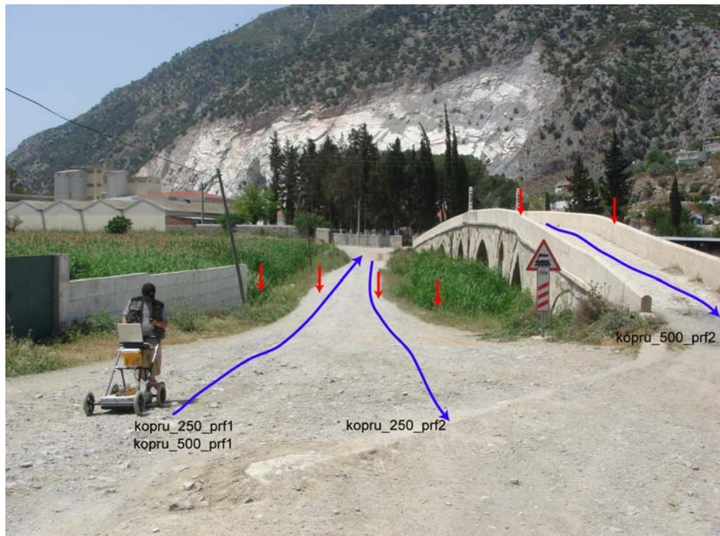
Figure 4.20: Location of GPR profiles (blue lines correspond to GPR profiles and red arrows indicate the possible fault zone).
