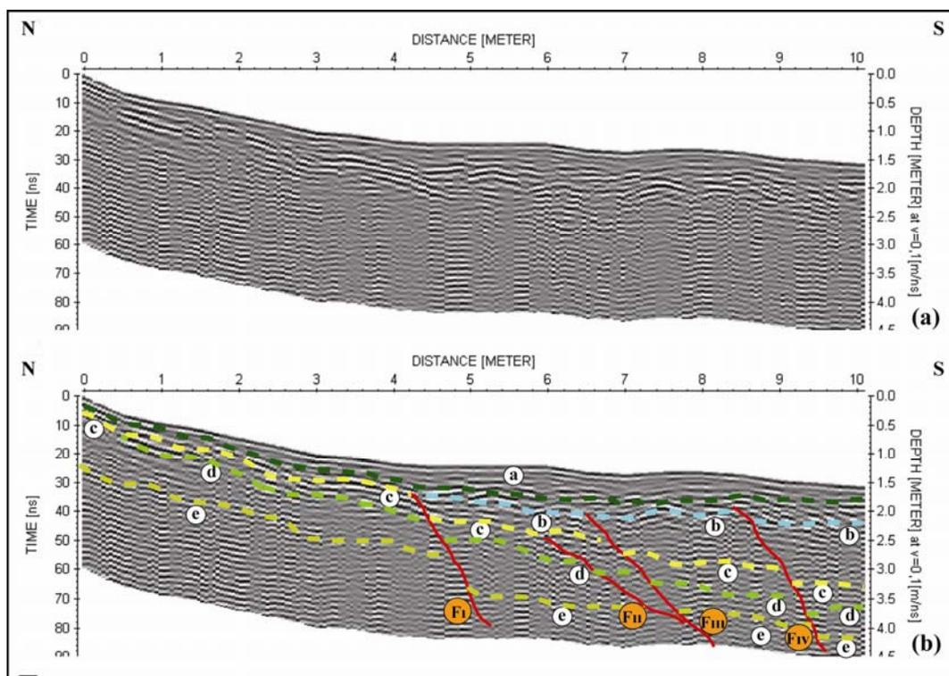
*Figure 4.6: 500 MHz GPR profile in the Argavli trench site (a) Processed profile. (b) Interpreted profile. Dashed lines and the letters from “a” to “e” represent 5 different layers, thin red line and F<sub>I</sub> – F<sub>IV</sub> represents possible fault zones.*
