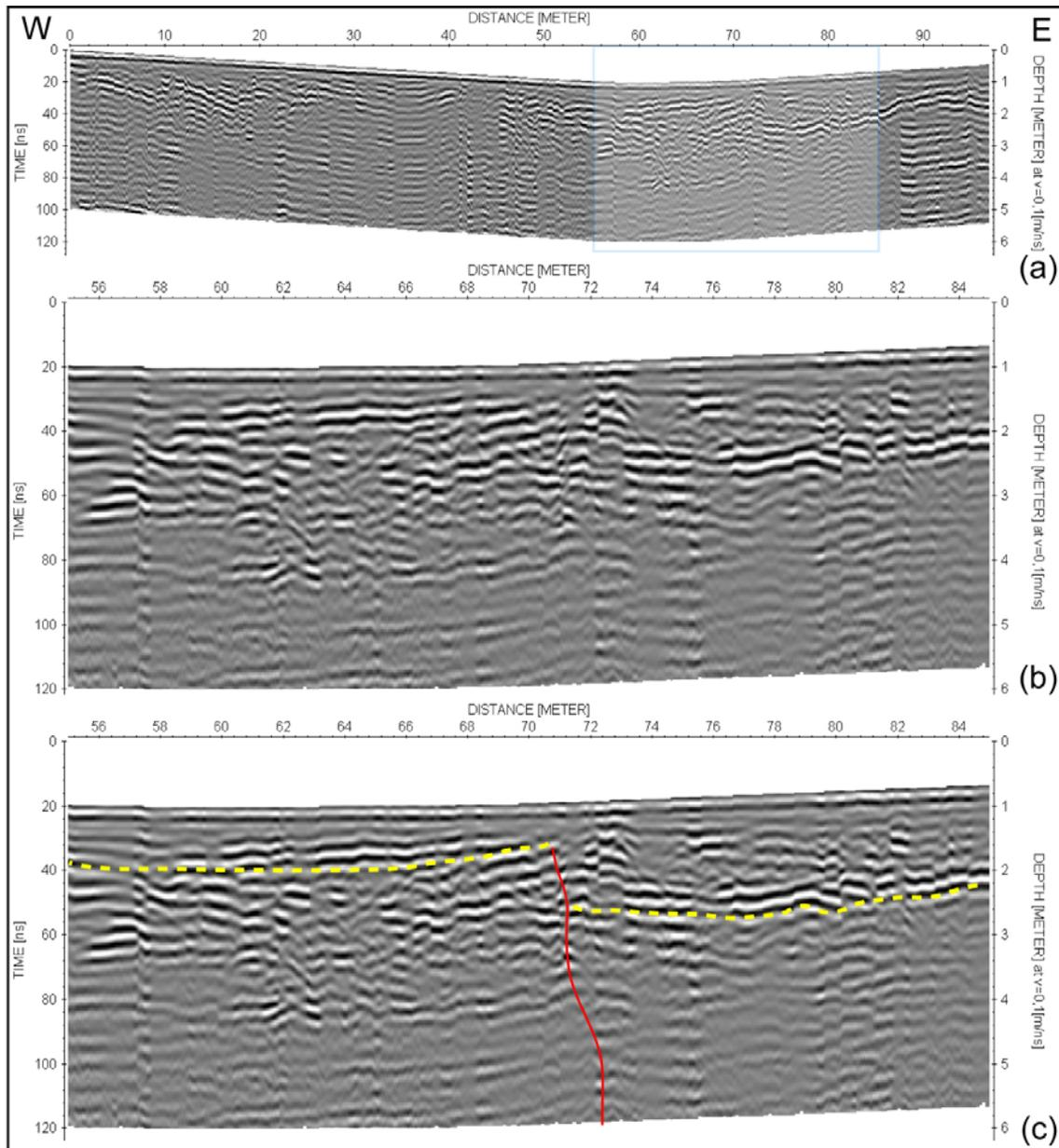
Figure 4.22: (a) Processed data of “kopru\_250\_prf2” GPR profile. (b) Zoomed on between 55 – 85 meter in highlighted square in “a”. (c) Interpretation of “kopru\_250\_prf2” GPR profile. Dashed lines represent the layers, thin red line represents possible fault zone.
