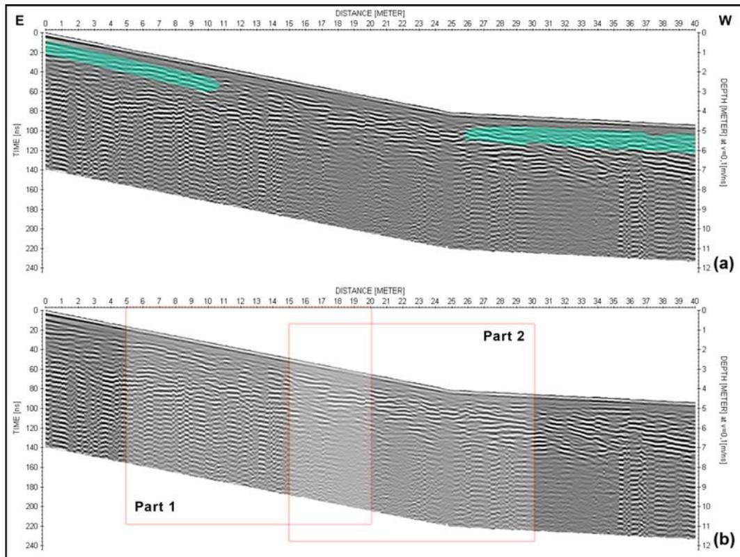
Figure 4.38: 250 MHz antenna profile of Roman Road. (a) Processed data of “roma\_road\_250\_prf1” GPR profile (blue highlighted areas represent high contrast reflectors). (b) Two interpreted detailed area of the profile (Part 1 and Part 2).
