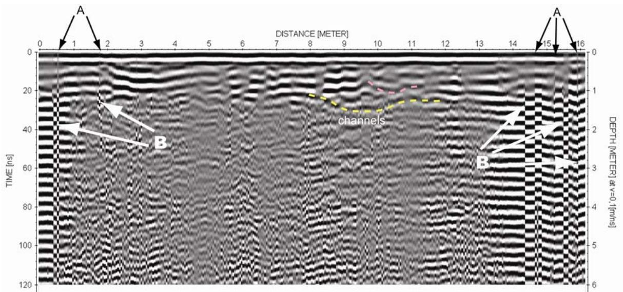
*Figure 2.8: A sample GPR profile for showing antenna coupling loss (arrows represent with “A” indicate un-even ground and clumps of vegetation and arrows represent with “B” indicate anomalous amplitude changes).*
