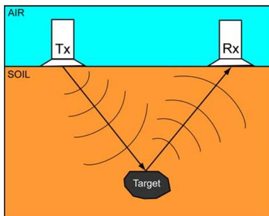
*Figure 2.1: Schematic view of GPR antennas working system.*
