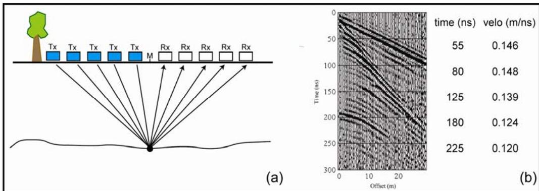
Figure 2.6: GPR acquisition using the common midpoint antenna configurations. (a) Schematic diagram view of common midpoint acquisition. (b) An example GPR section acquired using common midpoint (example GPR section redrawn from Travassos and Menezes 2004).
