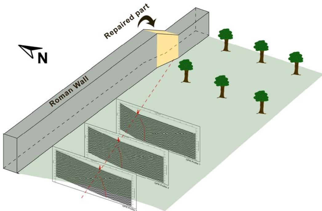
*Figure 4.33: The schematic view of the wall with the GPR profiles and possible fault zone (red arrows indicate the disturbed zone in the GPR profiles, red dashed line represents the possible fault zone and yellowish part of the wall was repaired).*
