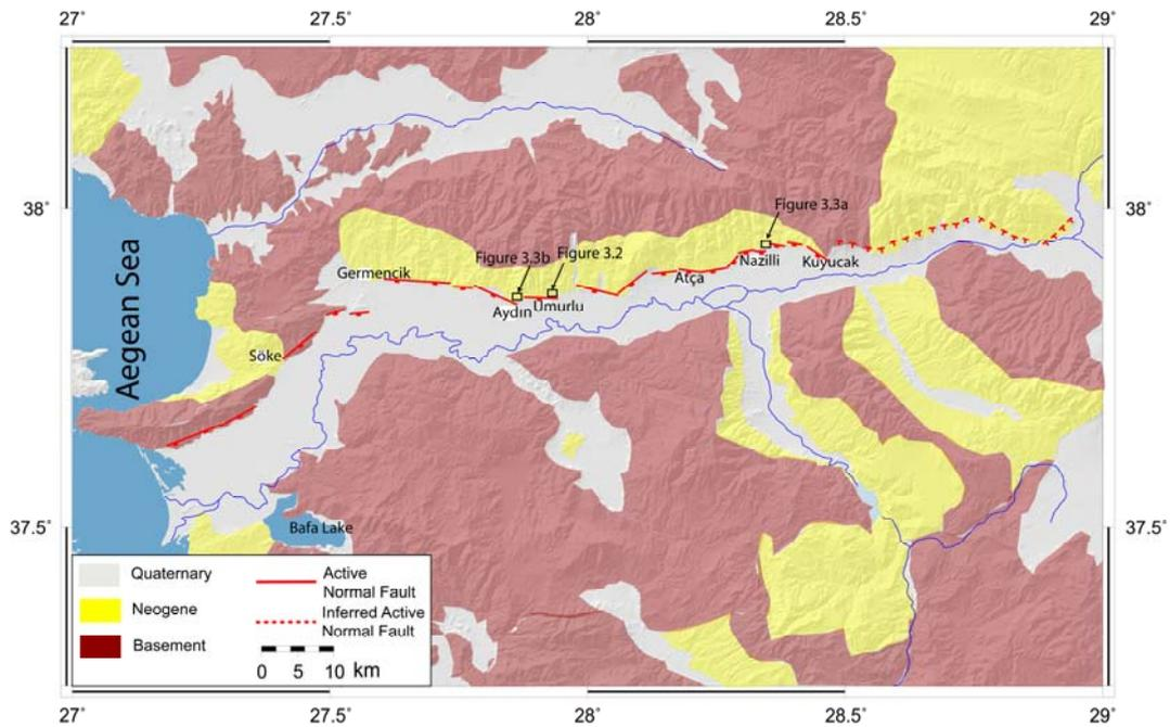
Figure 3.1: Simplified geological map on elevation map of the Büyük Menderes Graben showing general geological units (MTA 1/500.000 geological map of Turkey).
