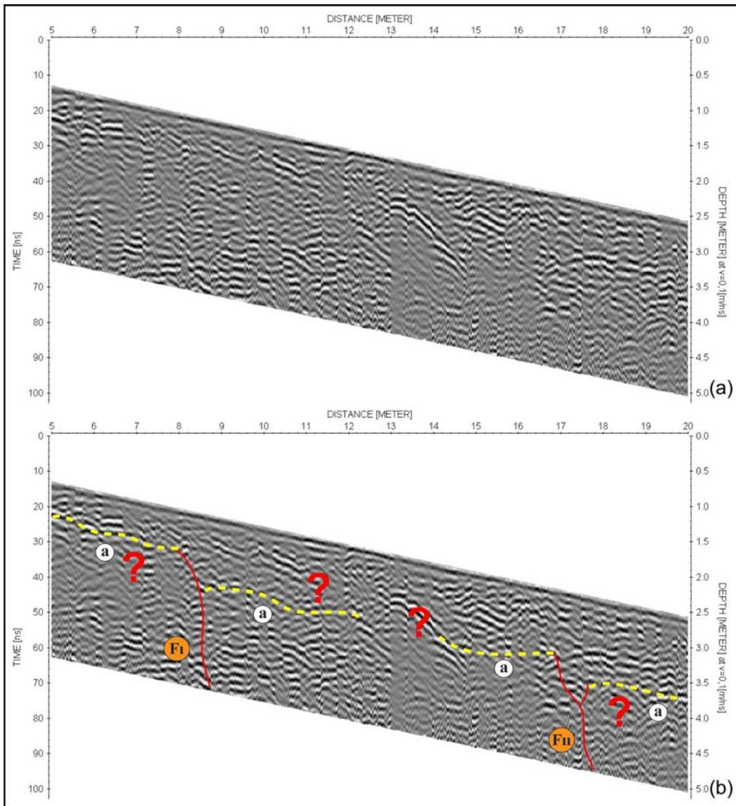
Figure 4.42: (a) Zoom view of the part 1 in Figure 4.41b. (b) Interpretation of the part 1. Dashed lines and letter "a" represent the layer and thin red line with "F1" and "F11" represent possible fault zone.
