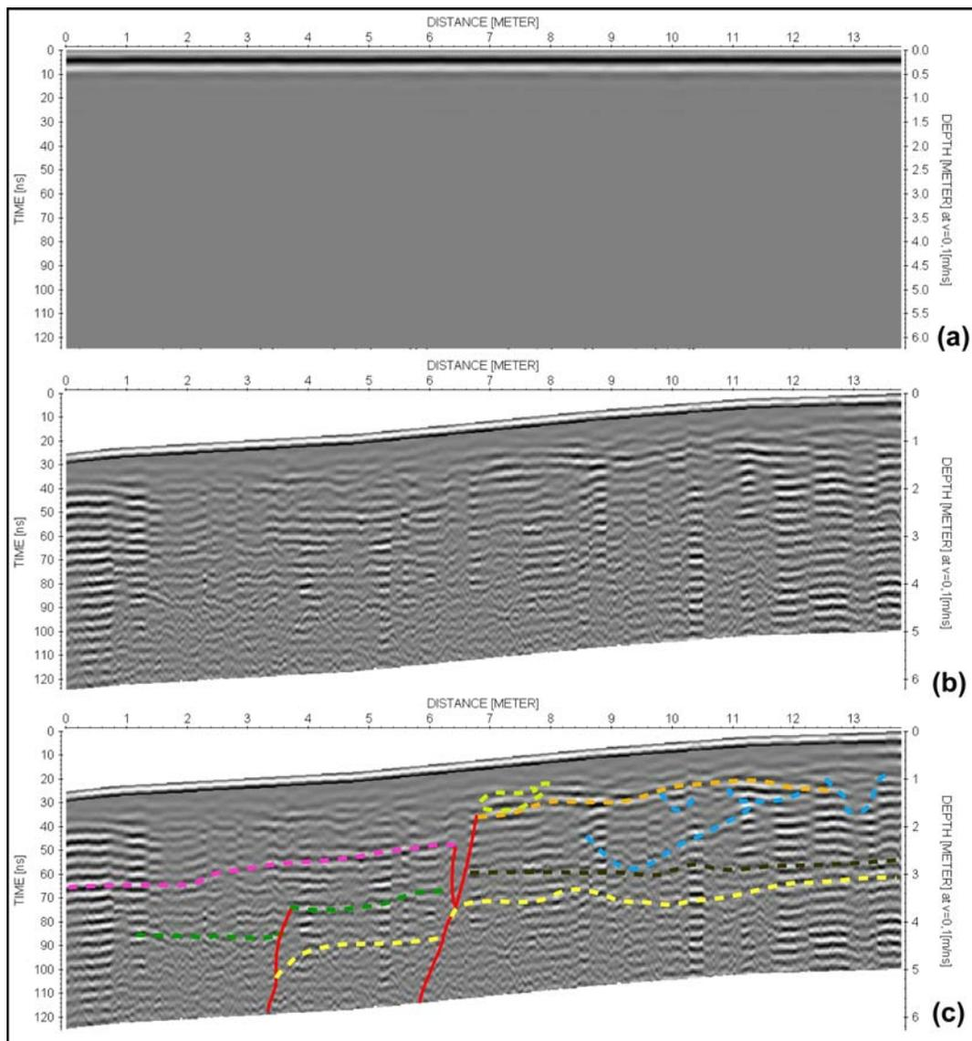
Figure 4.13: (a) Raw data of “atca\_250\_prf3” GPR profile. (b) Final section of “aca\_250\_prf3” GPR profile. (c) Interpretation of “atca\_250\_prf3” GPR profile. Dashed lines represent the layers, thin red line represents possible fault zone.
