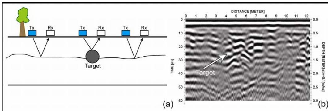
Figure 2.5: GPR acquisition using the constant offset antenna configurations. (a) Schematic diagram view of constant offset acquisition. (b) An example GPR section acquired using constant offset.
