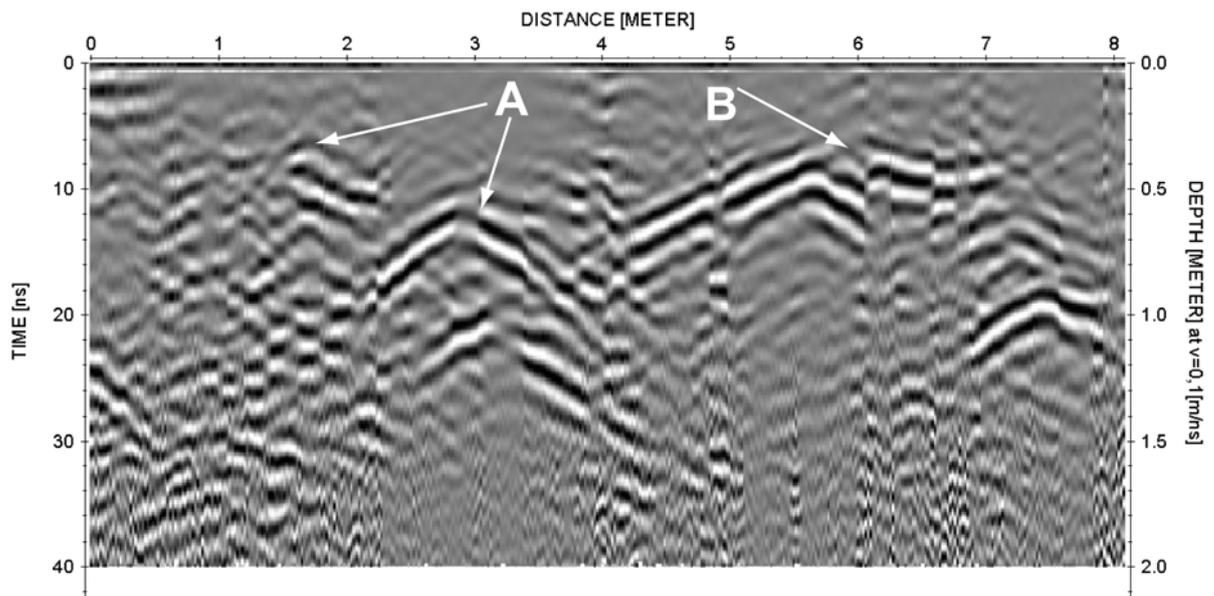
*Figure 2.10: A sample GPR profile for showing point source hyperbolas. Point source hyperbolas (A) are generated from buried objects of a limited size. In this case the hyperbola on the right was generated from a metal pipe and the lower amplitude hyperbola on the left from a plastic pipe. The series of high amplitude reflections that are stacked vertically at location B were generated by a large piece of metal near the ground surface.*
