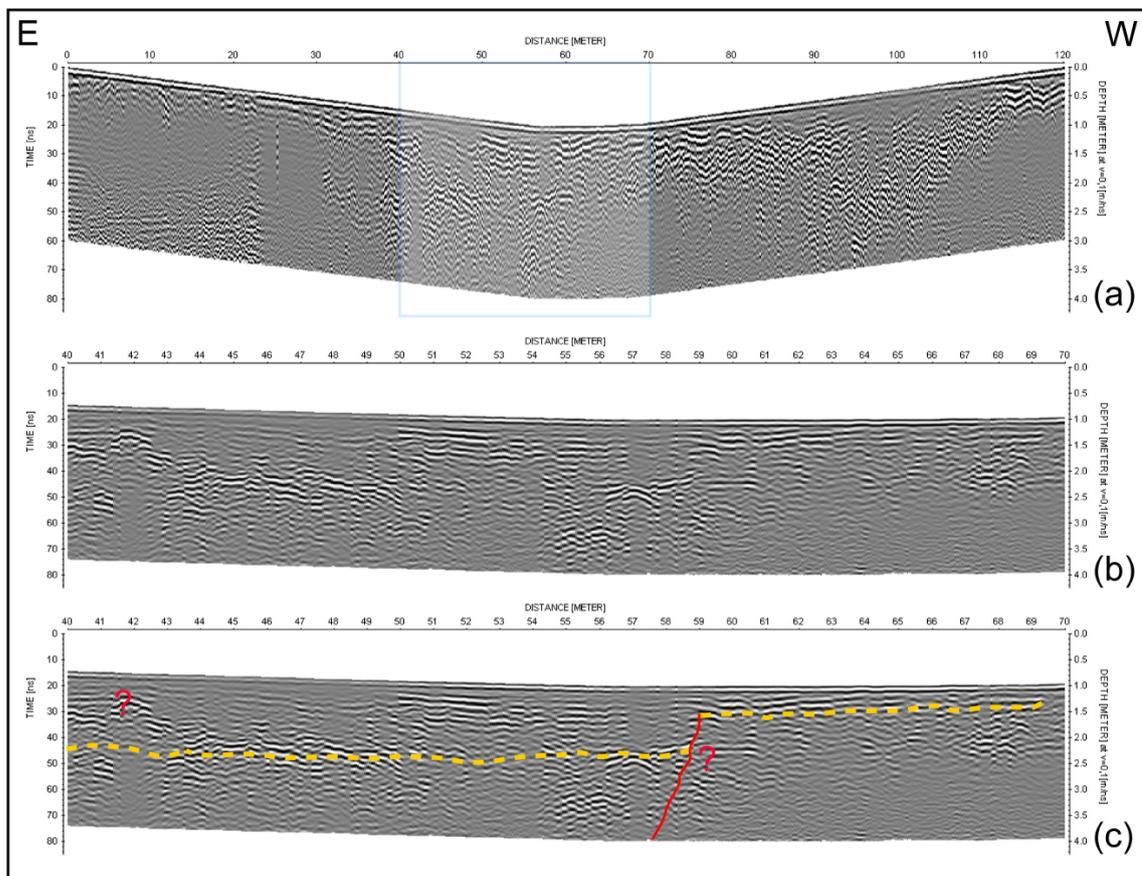
Figure 4.23: (a) Processed data of "kopru\_500\_prf1" GPR profile. (b) Zoomed on between 40 – 70 meter in highlighted square in "a". (c) Interpretation of "kopru\_500\_prf1" GPR profile. Dashed line represents the layers, thin red line represents possible fault zone.
