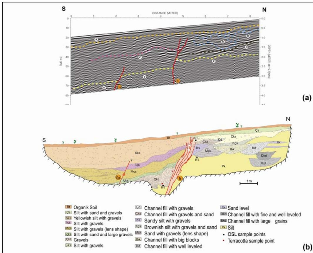
Figure 4.16: Comparison of the 500 MHz GPR profile (a) with the trench log (b). Both figures are in the same scale and no vertical exaggeration
