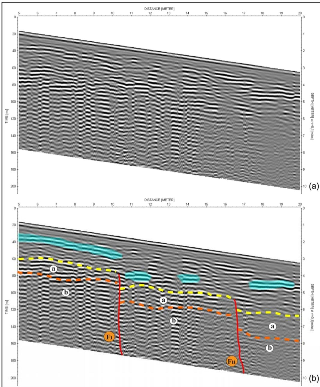
Figure 4.39: (a) Zoom view of the part 1 in Figure 4.38b. (b) Interpretation of the part 1. Blue highlighted areas represent high contrast reflectors, dashed lines and letters "a" and "b" represent the layers and thin red line with "F1" and "F2" represent possible fault zone.
