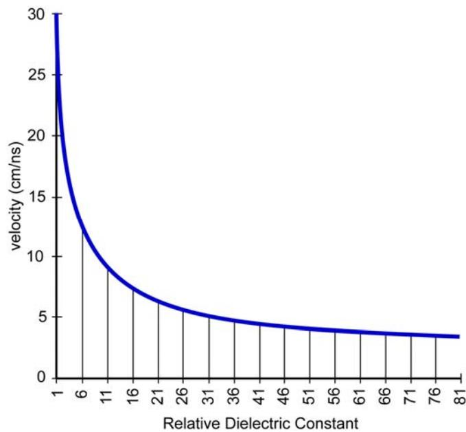
Figure 2.2: Relation between velocity and relative dielectric constant (Daniels, 2004).
