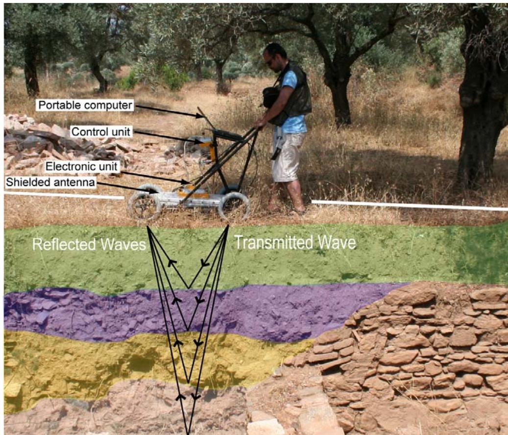
Figure 2.7: Collecting GPR data with 250 MHz shielded antenna with constant offset (Commercial Mala Geoscience Ramac GPR system).
