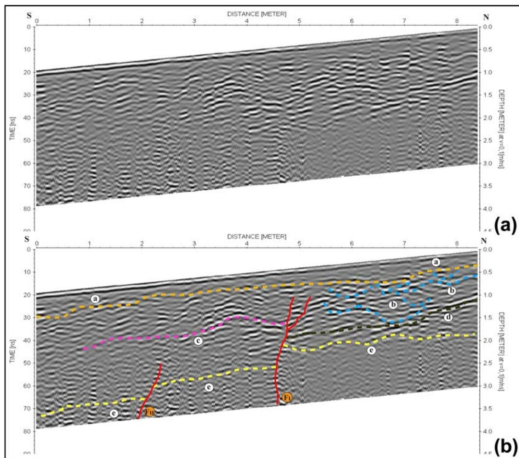
Figure 4.14: (a) Processed data of “atca\_500\_prf2” GPR profile. (b) Interpretation of “atca\_500\_prf2” GPR profile. Dashed lines and the letters from “a” to “e” represent 5 different layers, thin red line and F<sub>1</sub> & F<sub>11</sub> represents possible fault zones.
