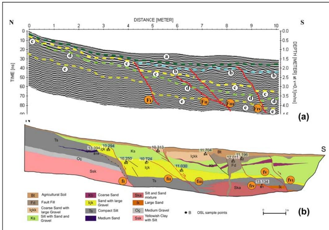
Figure 4.8: Comparison of the 500 MHz GPR profile (a) with the trench log (b). Both figures are in the same scale and no vertical exaggeration.
