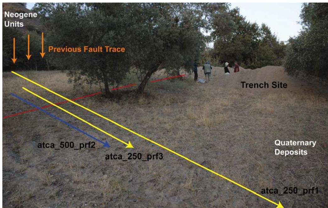
Figure 4.10: GPR profiles and trench location illustration on the site photo. Red thin line indicates active fault and brown arrows indicate previous fault trace between Neogene units and Quaternary deposits (looking towards northwest).
