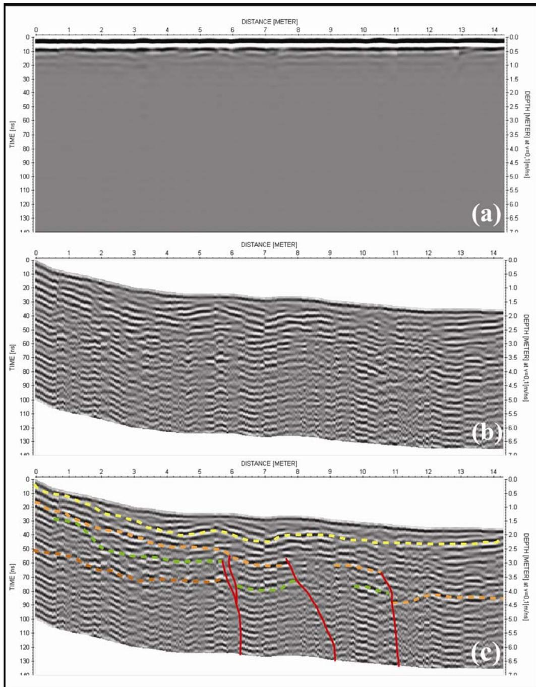
Figure 4.5: 250 MHz GPR profile in the Argavlı trench site. (a) Raw profil, (b) Processed profile, (c) Interpreted profile. Dashed lines represent the layers, thin red line represents possible faults.
