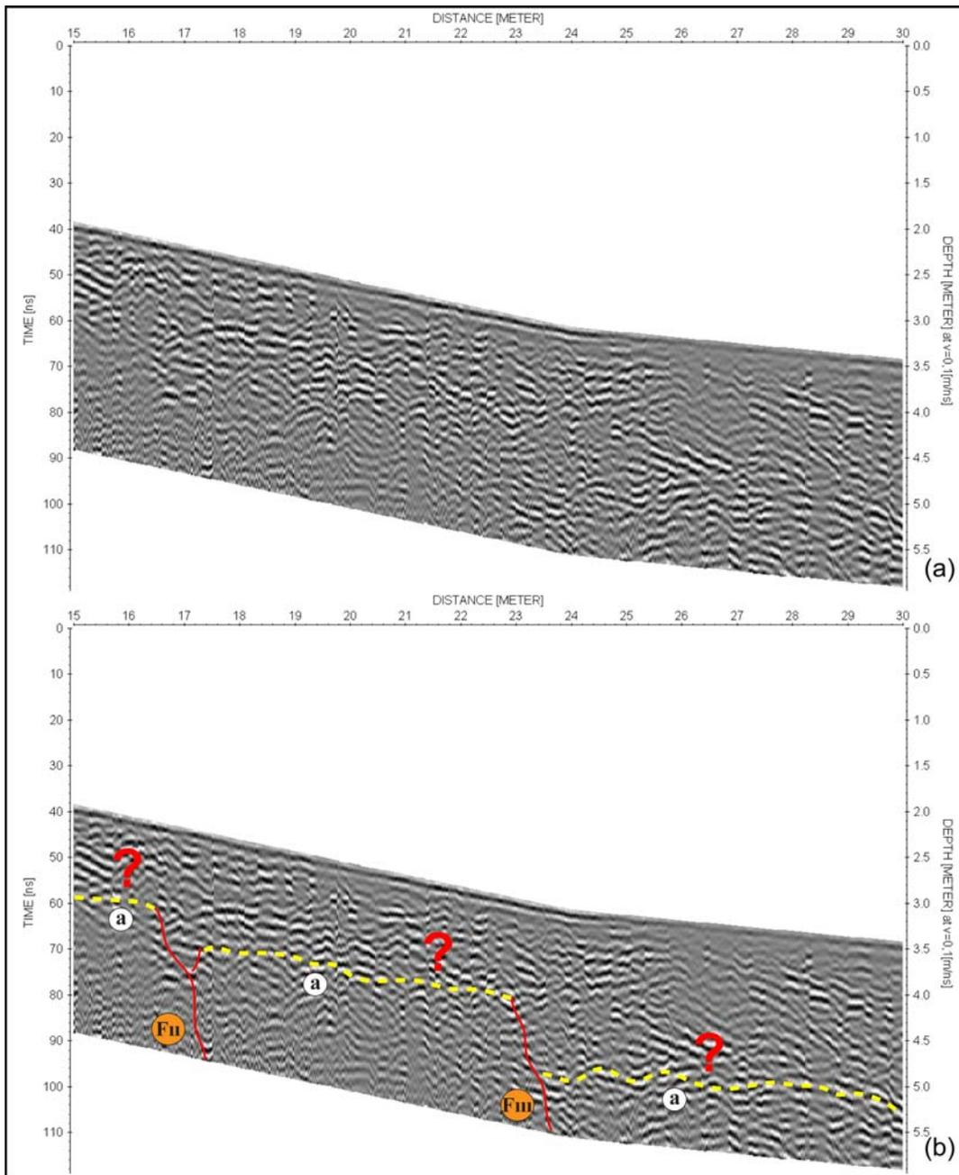
Figure 4.43: (a) Zoom view of the part 2 in Figure 4.41b. (b) Interpretation of the part 2. Dashed lines and letter "a" represent the layer and thin red line with "F1" and "F2" represent possible fault zone.
