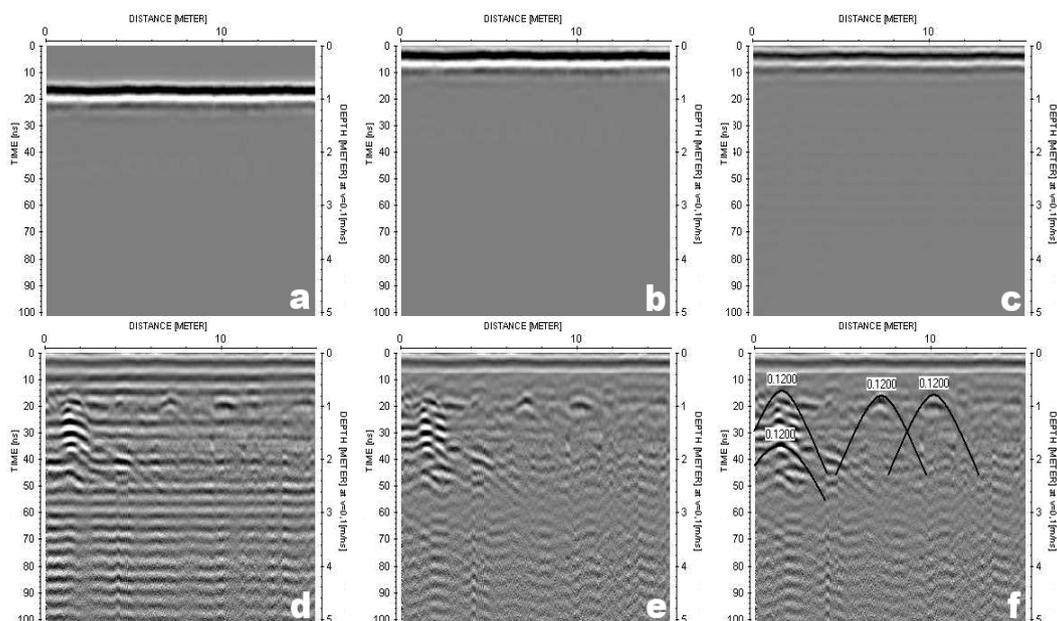
Figure 2.11: An example GPR profile and its processing steps. (a) Raw data. (b) After filtered with move starttime. (c) After filtered with subtract-mean (dewow). (d) After filtered with energy decay. (e) After filtered with subtracting average. (f) After velocity analysis with the diffraction hyperbolas method.
