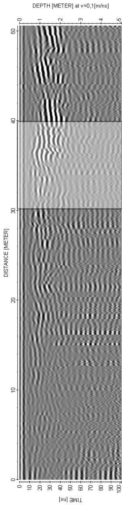
Figure 4. 12: 250 MHz antenna profile (atca\_250\_prf1 in Figure 4.10). Highlighted area indicates the location of anomalous zone.
