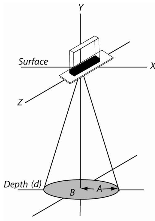
Figure 2.4: Approximate GPR-antenna footprint (Fresnel zone) for bistatic, dipole antennas (adapted from Martinez and Byrnes, 2001). This footprint is calculated using Equation (1).  $A$  = long radius;  $B$  = short radius;  $Y$  = elevation, where  $X$  is the surface elevation and  $d$  is the depth of the Fresnel zone.
