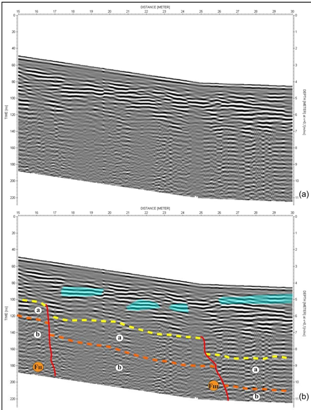
Figure 4.40: (a) Zoom view of the part 2 in Figure 4.38b. (b) Interpretation of the part 2. Blue highlighted areas represent high contrast reflectors, dashed lines and letters "a" and "b" represent the layers and thin red line with "F1" and "F11" represent possible fault zone.
