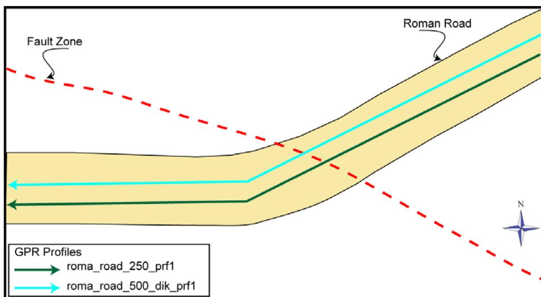
Figure 4.37: Unscale, schematic top view of the GPR profiles.
