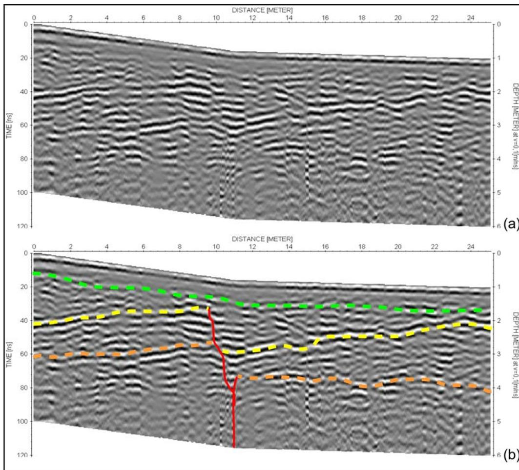
Figure 4.31: (a) Processed data of "GPR\_profile\_2" GPR profile. (b) Interpretation of "GPR\_profile\_2" GPR profile. Dashed lines represent the layers, thin red line represents possible fault zone.
