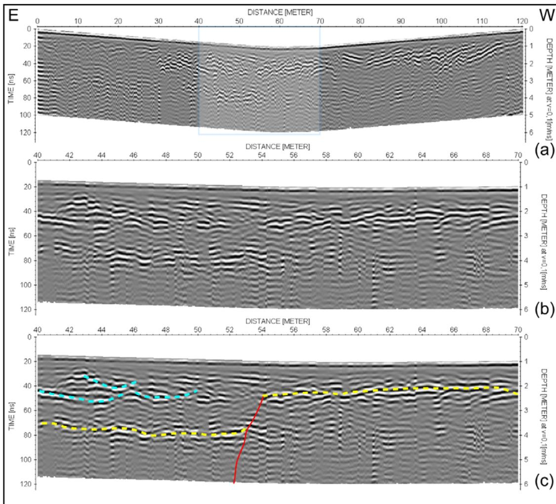
Figure 4.21: (a) Processed data of “kopru\_250\_prf1” GPR profile. (b) Zoomed on between 40 – 70 meter in highlighted square in “a”. (c) Interpretation of “kopru\_250\_prf1” GPR profile. Yellow dashed line represents the layer, blue dashed lines represent channel fills and thin red line represents possible fault zone.
