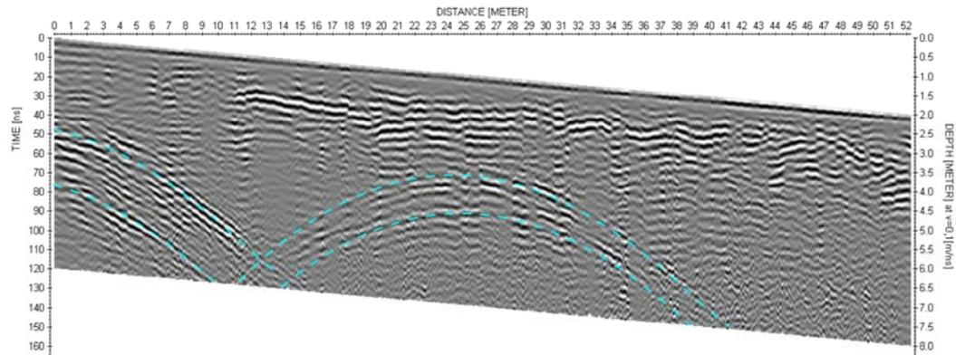
Figure 2.14: GPR data with modeled diffractions from the surface scatterers (light blue hyperbolas) superimposed. With a velocity of 0.3 m/ns was used.
