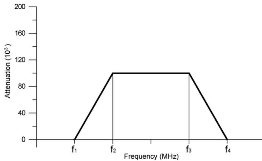
Figure 2.13: Schematic description of bandpass frequency filter.
