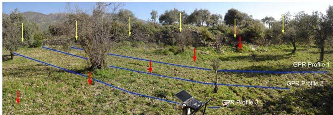
Figure 4.28: Picture shows the position of the wall (yellow arrows), fault zone (red arrows) and GPR profiles (blue lines) (looking towards NE).
