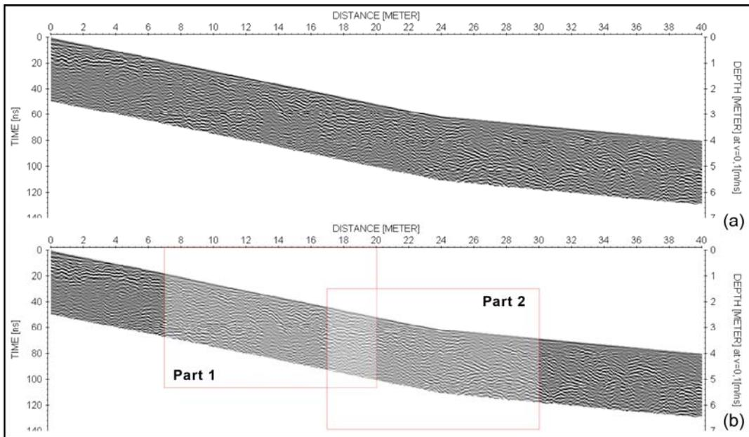
Figure 4.41: (a) Processed data of "roma\_road\_500\_prf1" GPR profile. (b) Two interpreted detailed area of the profile (1. region and 2. region).
