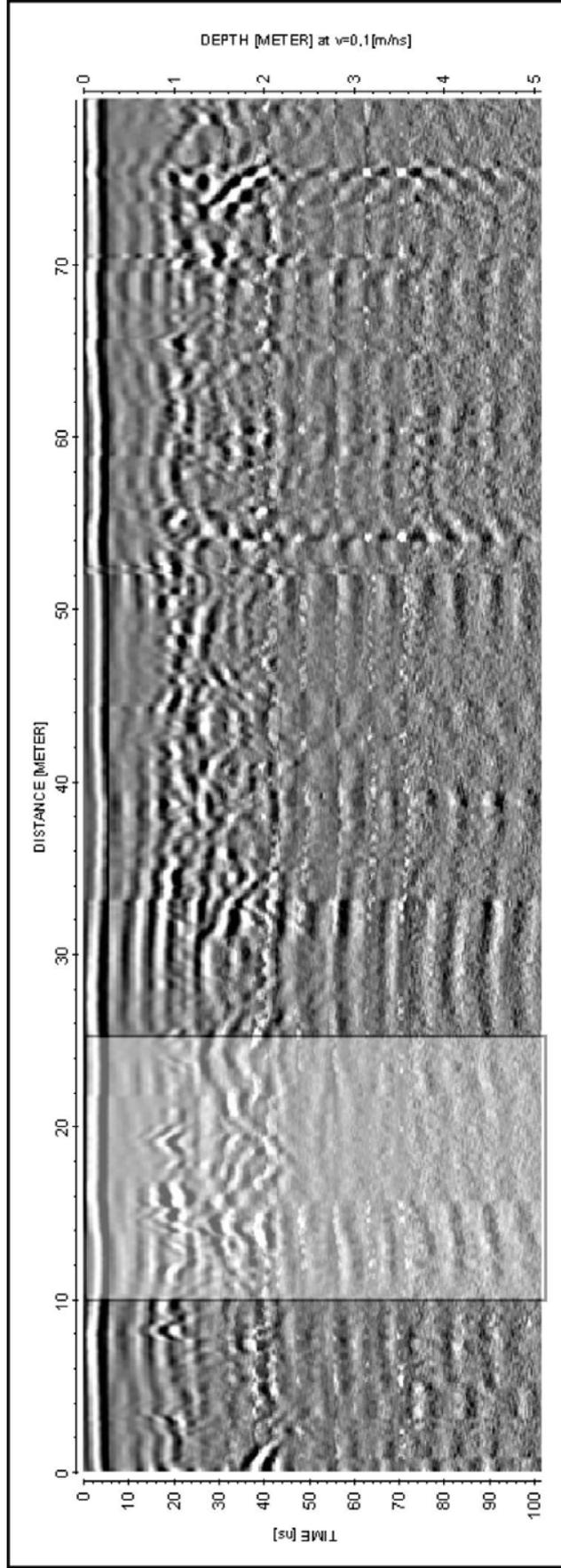
Figure 4. 4: 250 MHz antenna profile (argavl\_250\_prf1 in Figure 4.4). Highlighted area indicates the location of anomalous zone.
