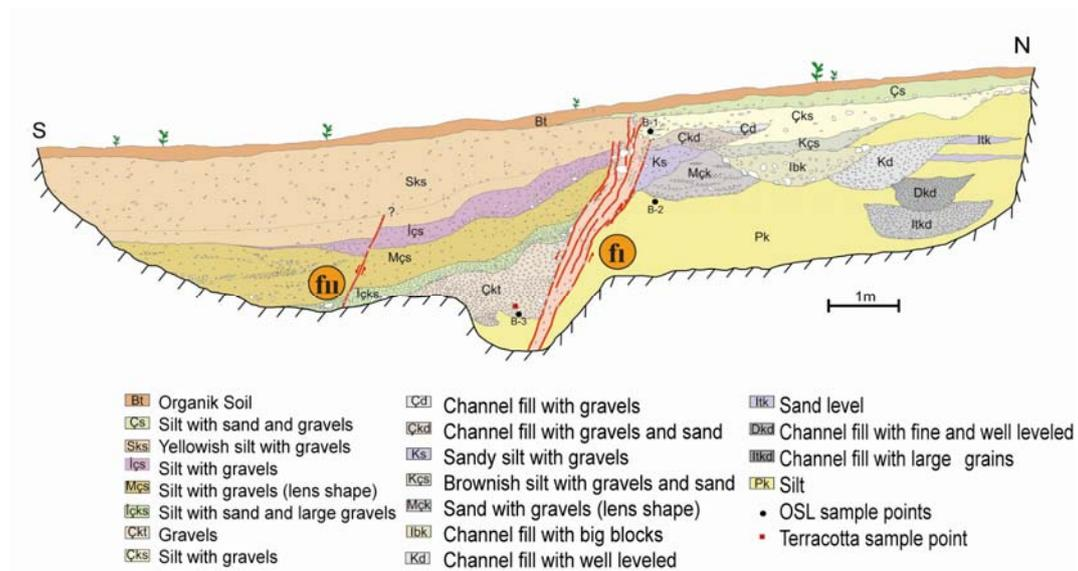
Figure 4.15: Trench exposure for eastern wall of Argavlı. Trench walls are drawn with no vertical exaggeration. (main faults marked as “*fi*” and “*fi*<sub>1</sub>”) (Altunel *et al.*, 2009).
