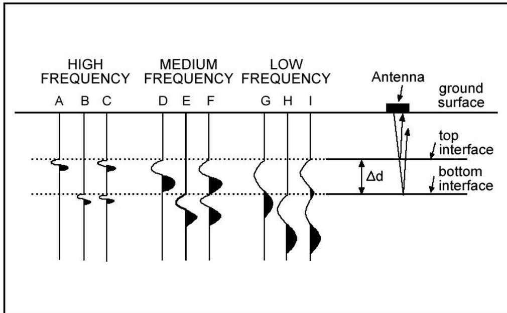
Figure 2.3: Schematic view of GPR trace between two planar interfaces (Redrawn from Conyers, 2004).
