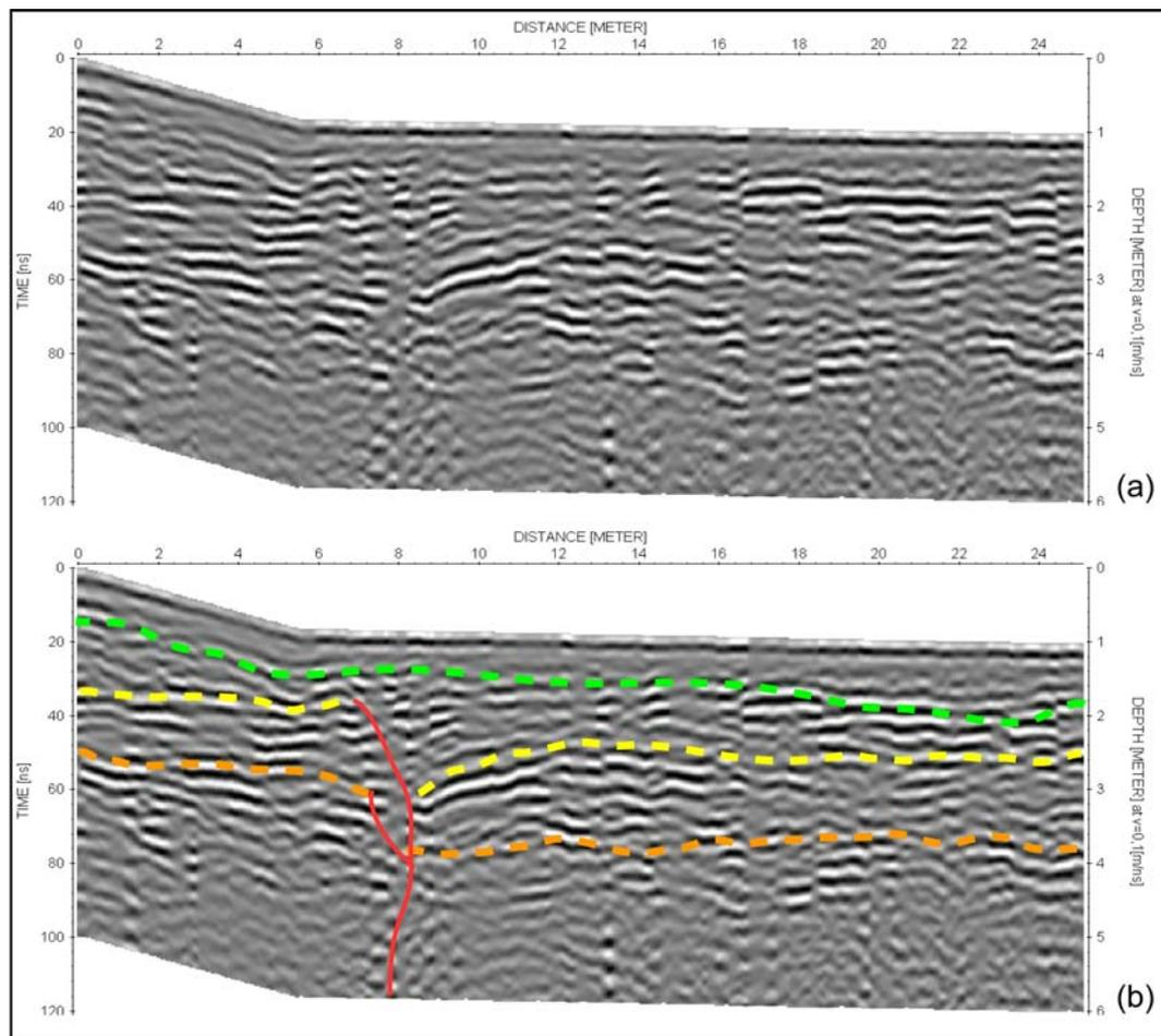
Figure 4.30: (a) Processed data of "GPR\_profile\_1" GPR profile. (b) Interpretation of "GPR\_profile\_1" GPR profile. Dashed lines represent the layers, thin red line represents possible fault zone.
