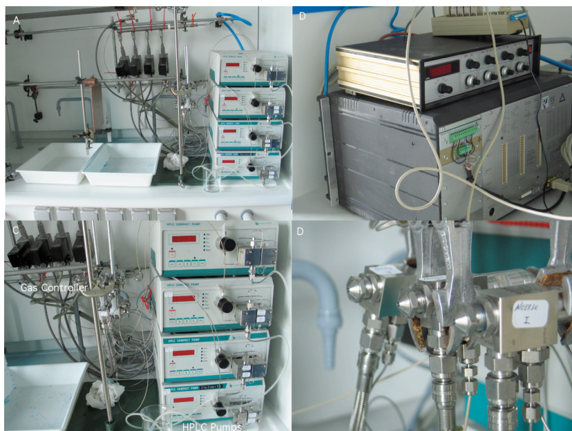
Figure 3: Simultaneous spray machine (A) General set up (B) Central control unit (C) HPLC pumps and gas controller and (D) zoomed spray nozzles
