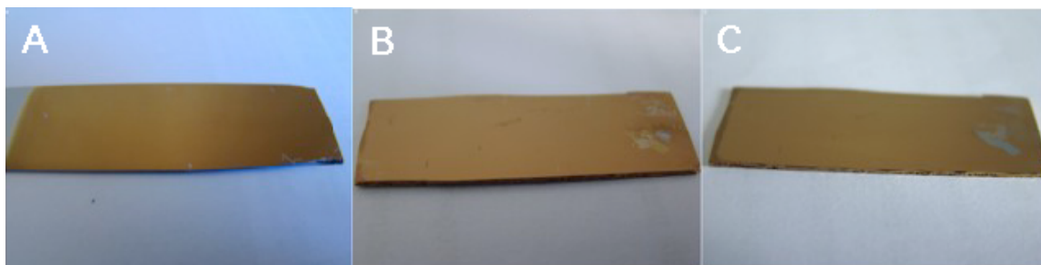
Figure 26: Optical micrograph of (A) dipped (PAH/Au NP) 20 film, (B) sprayed (PAH/Au NP) 40 film and (C) sprayed (PAH/Au NP) 50 film
