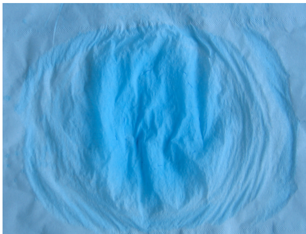
Figure 10: Approach used for spray nozzle alignment using a colored liquid
