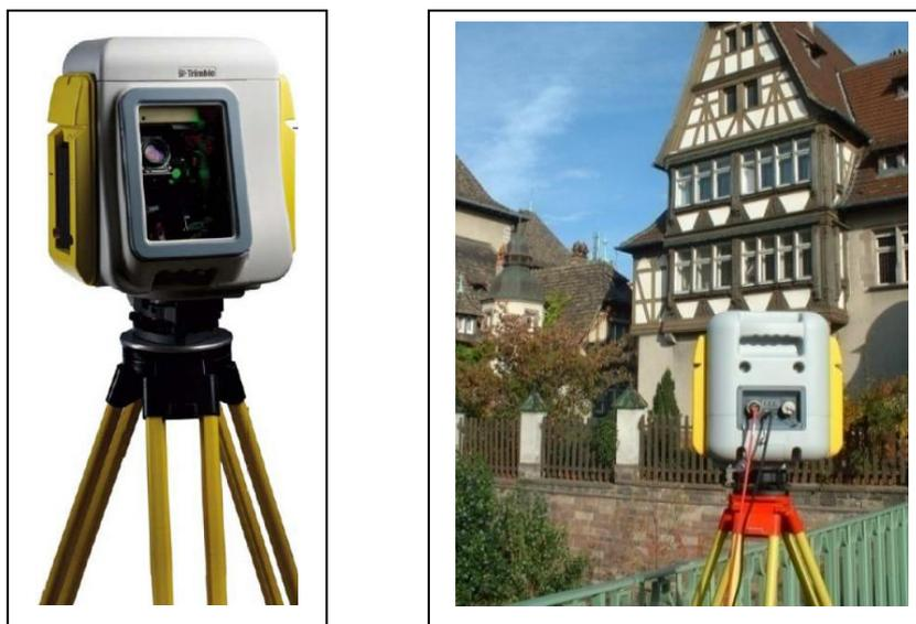
Figure 3.2. Scanner laser Trimble GX
