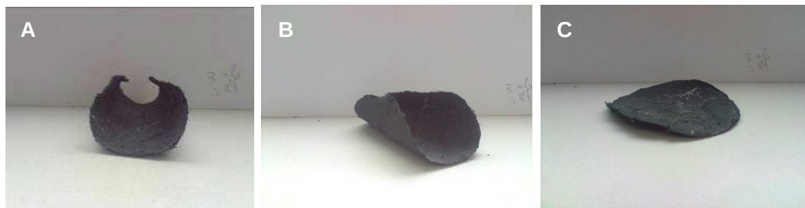
Figure 2. The optical photos of VA-CNTs made BP with high flexibility and complete shape recovery after its bending.
