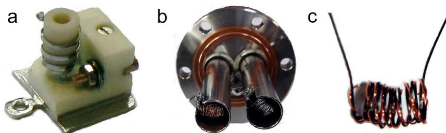
Figure 1.5: Homebuilt evaporators: a) molecular evaporator. The substance powder is held by a ceramic crucible and evaporated by means of Joule heating through a wiled tantalum filament. b) multiple-metal evaporator. The metal wire is wound around a tungsten filament [shown in (c)]. By means of joule heating small amounts of atoms can be evaporated, the shielding tubes preventing cross-contamination of the filaments.
