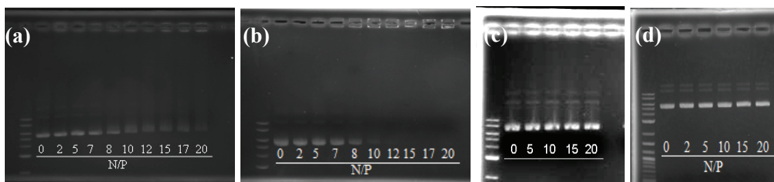
Figure 3.11. Agarose gel electrophoresis (0.9 %) of a) DPTA-C12-C8-G , b) Orn-C8-C12-G , c) DPTA-C12-C8-L and d) Orn-C8-C12-L complexed with pDNA at different N/P ratios. Band on the left of each gel corresponds to 10 kb DNA ladder. The final pDNA (phosphate) concentration was 60 \mu M, while the bola concentration was varied to obtain the final N/P ratio.
