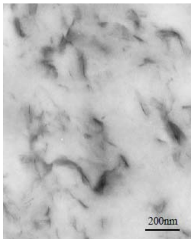
Figure 140 : Image TEM de films nanocomposites LNP3
