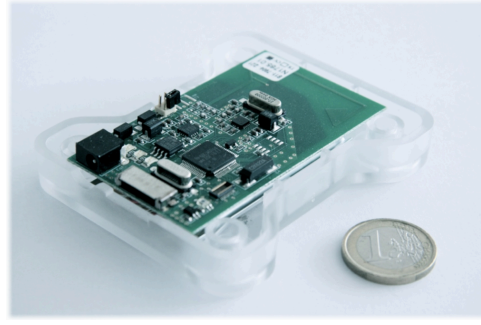
Figure 1: An example of wireless sensor node: the WSN430 [87]
