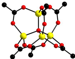
Fig. 42: Structure of the tetrahedral core in [\text{Zn}_4\text{O}(\text{BDC})_3] (MOF-5).
