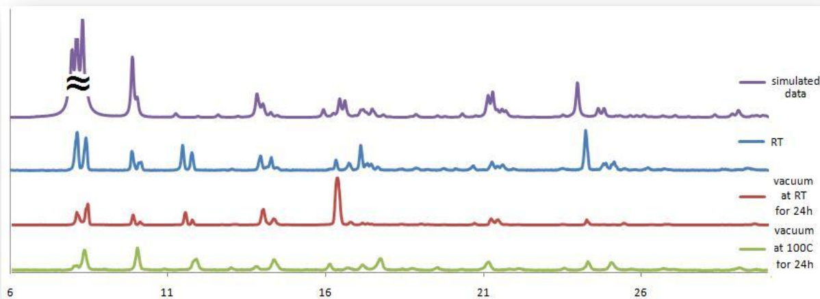
Fig. 66: Powder X-ray diffraction analyses of 18 after the desolvation in different conditions.
