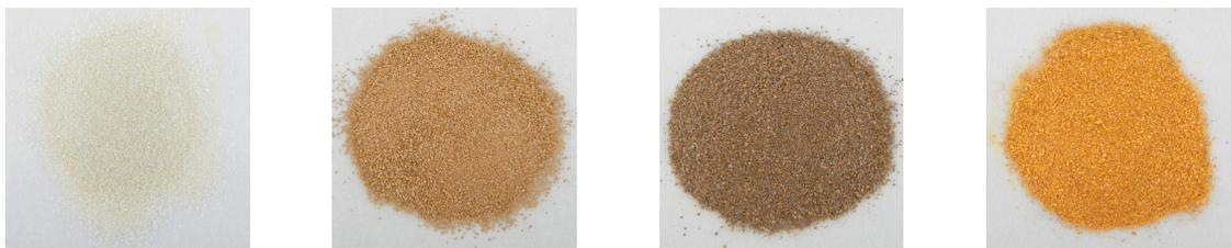
**Figure 5.10** From left to right: Photos of ammonium metavanadate and the decomposition products after heating to 190°C, 270°C and 325°C.
