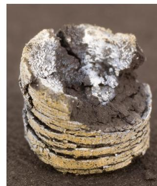
**Figure 6.11** Macro photograph of the residue of a  $\text{MnO}_x\text{@CNF/Al}$  pellet after combustion.
