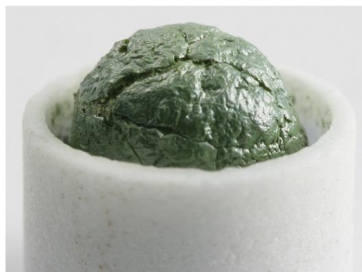
**Figure 5.7** Photo of a “dome” of  $\text{Cr}_2\text{O}_3$  foam obtained by thermogravimetric analysis of chromium nitrate, residue from the test in Figure 5.5.
