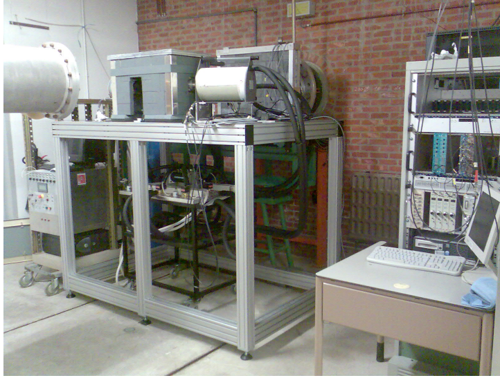
Figure 3.4: Picture of the experimental setup showing the lead shielding as well as the different HPGe detectors on the table in the left and the data acquisition system in the right.
