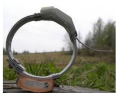
Fig 3.2: GPS/Argos collar of brand ES-PAS (Moscow, Russian Federation). Size: 205x50 mm (HxL), neck size: 37-42cm, weight: 500g.
