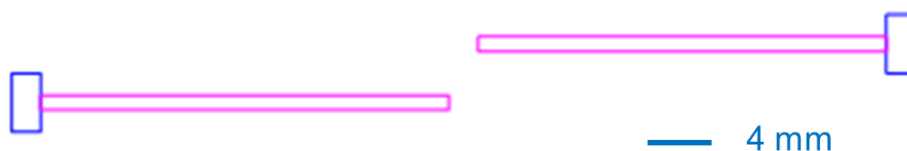
Figure B.2 AutoCAD drawing of the ‘Dropslot’ emulsion analysis chip. Pink channels are: 25 \mu\text{m} deep, blue channels are 260 \mu\text{m} deep.
