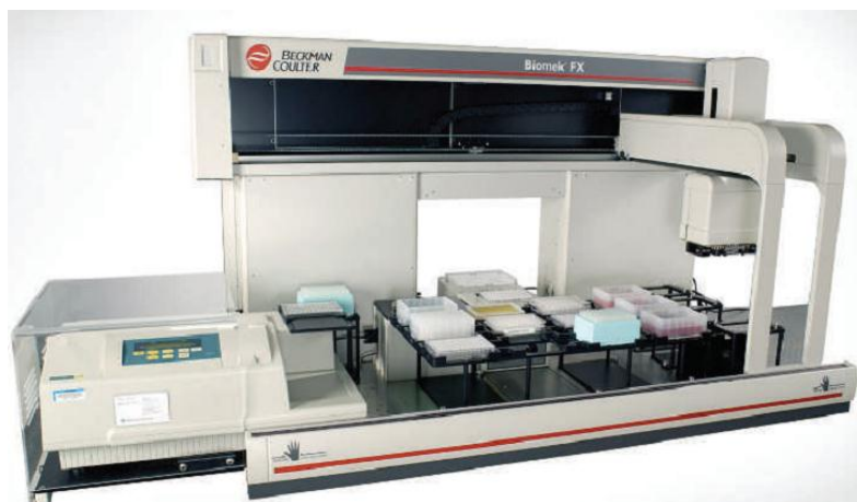
Figure 1.1 Example of an automated HTS platform using microplates. Operations performed include plate storage, incubation, reading on a fluorimeter and washing. Picture taken from ref [2].
