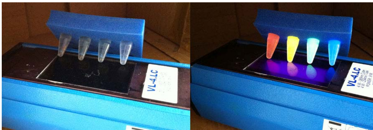
Figure 7.21. Fluorescence solvatochromism of 3-methoxychromone derivative (compound 44).
