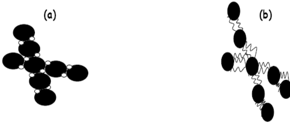
Figure III. 6: Difference of microstructure aggregate before (a) and after (b) deformation.
