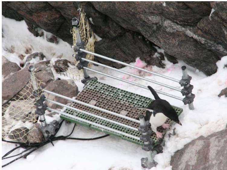
Figure IV - 12: Adélie penguin on the weighbridge. The bridge has to be snow-free to measure correct weights and is checked every day. The three scales in a row can be seen on this picture.
