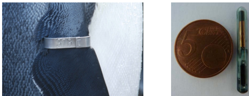
Figure IV - 1: Stainless steel flipper band (on the left) and transponder tag (on the right).
