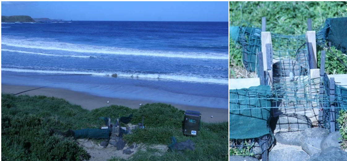
Figure IV - 11: Phillip Island weighbridge. The weighbridge is situated between the sea and the colony on an obligate path of the penguins.
