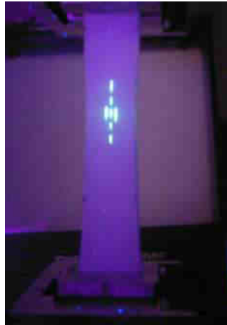
Figure III-4: Monitoring of markers printed on a tensile specimen by means of VidéoTraction extensometer
