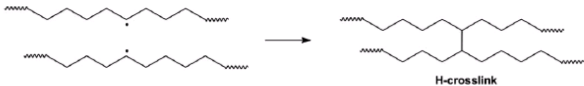
Figure II-16: The phenomenon of cross-linking [16]
