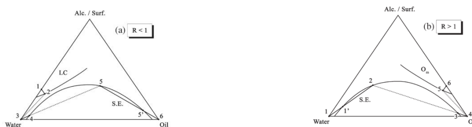
Fig.4. Diffusion path of water/alcohol+surfactant/oil system. (a) Hydrophilic surfactant ( R > 1 ). Segment (2-3), aqueous sub-phase. Segment (5-5'), spontaneous emulsification region. (b) Hydrophobic surfactant ( R < 1 ). Segment (1'-2), spontaneous emulsification region 6 .
