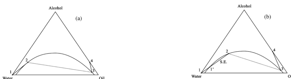
Fig.3. Ternary diagram of water/alcohol/oil system. Segment (1-2), diffusion path of aqueous phase. Segment (3-4), diffusion path of oily phase. Segment (2-3), interfacial local equilibrium. (a) No spontaneous emulsification region. (b) Segment (1'-2), spontaneous emulsification region 6 .
