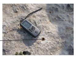
Figure III.6: Example of GPS monument used in Syria Thales DSNP 6502MK receivers and Leica AT504 Choke Ring Antenna
