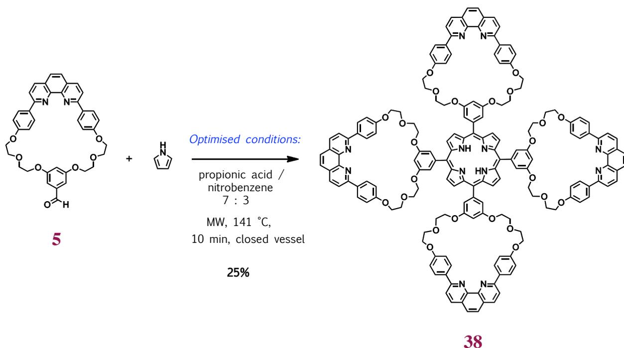
**Figure V.3.** Synthesis of tetra-substituted free-base porphyrin **38**. Optimised conditions for the condensation: **5** (1 eq., 200 mM), pyrrole (1 eq., 200 mM), propionic acid/nitrobenzene 7:3, microwaves, 141°C, 10 min (25%).
