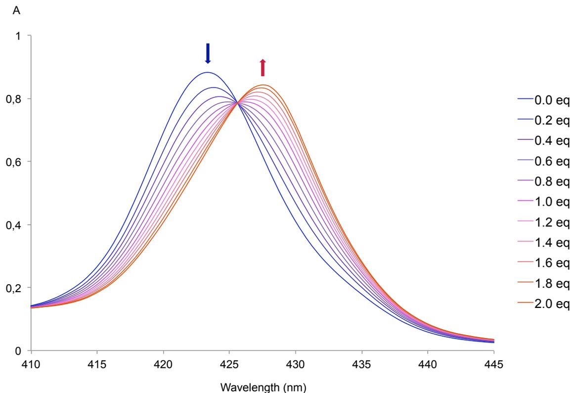
**Figure III.18.** UV-visible titration spectra in toluene (Soret band) of rotaxane **19**<sup>4+</sup> ( $0.92 \times 10^{-6}$  M) with 4,4'-bipyridine guest **G2** ( $2.8 \times 10^{-5}$  M) from 0.0 to 2.0 equiv. Arrows show changes in the host spectrum with increasing guest concentration; a 5 nm red shift from 423 to 428 nm is observed.
