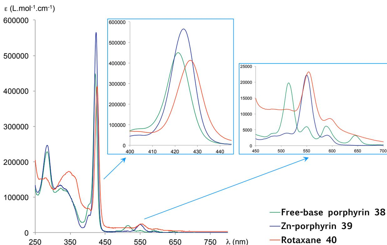
Figure V.10. UV-visible absorption spectra of free-base porphyrin **38**, Zn-porphyrin **39** and rotaxane **40<sup>4+</sup>** in  $\text{CH}_2\text{Cl}_2$ .
