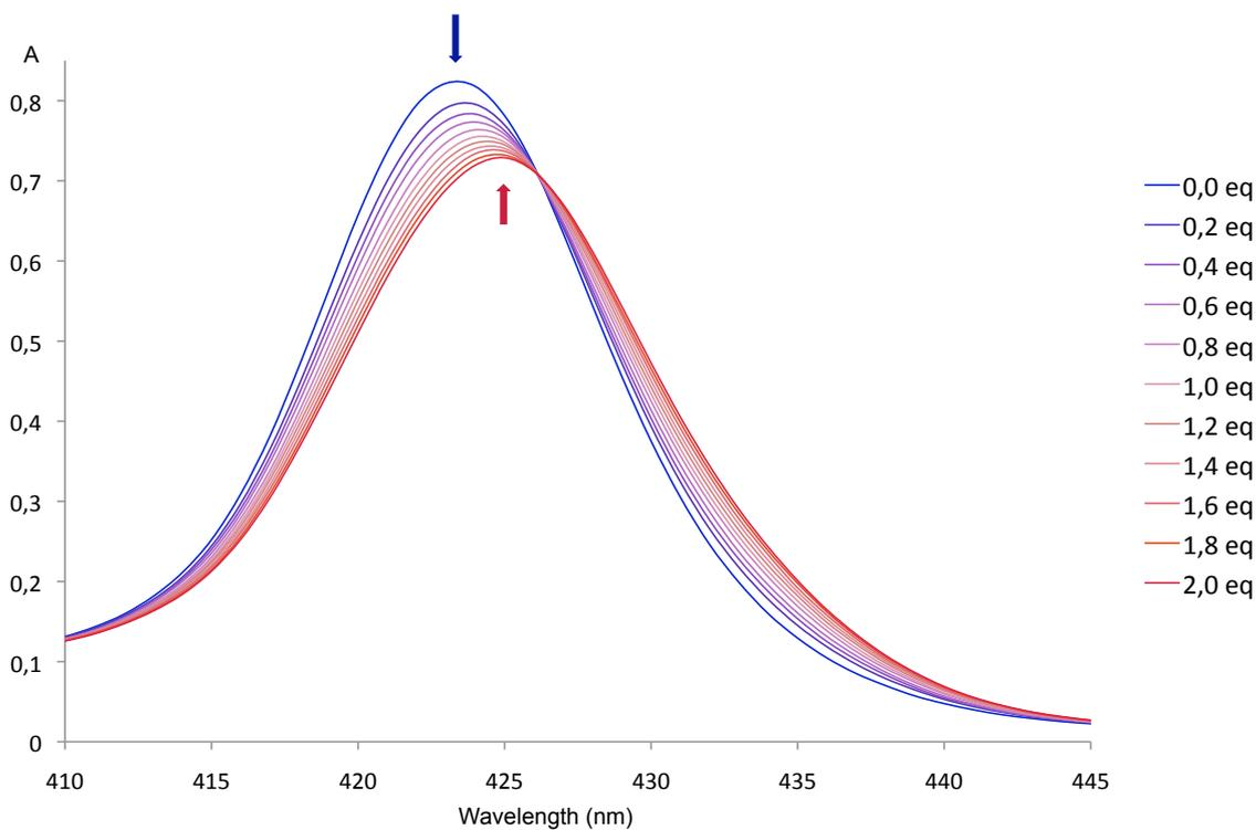
**Figure III.20.** UV-visible titration spectra in toluene (Soret band) of rotaxane **19**<sup>4+</sup> ( $0.92 \times 10^{-6}$  M) with guest **G3** ( $2.8 \times 10^{-5}$  M) from 0.0 to 2.0 equiv. Arrows show changes in the host spectrum with increasing guest concentration; a 2 nm red shift from 423 to 425 nm is observed.
