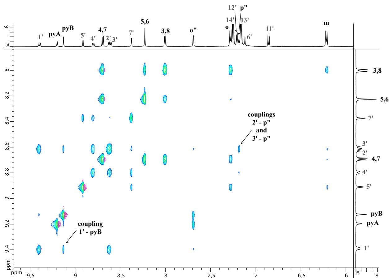
**Figure V.9.** Aromatic region of the <sup>1</sup>H-<sup>1</sup>H NOESY (600 MHz) spectrum of rotaxane **40<sup>4+</sup>**. NOE correlations between the rod and the tetra-macrocycle in the aromatic region are highlighted.
