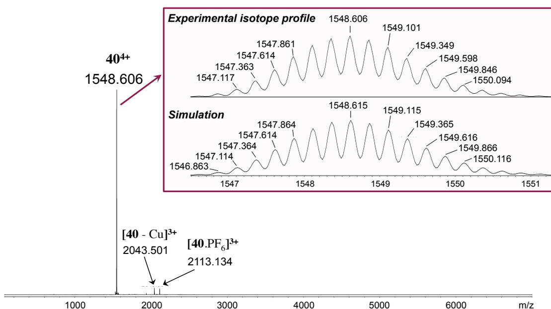
**Figure V.7.** HRES-MS spectrum of [3]rotaxane  $40^{4+}$  and isotope profile evidencing the 1:2 porphyrin/rod stoichiometry.
