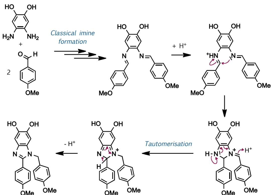
**Figure IV.16.** Possible mechanism for the formation of **33** in the presence of catalytic acid.
