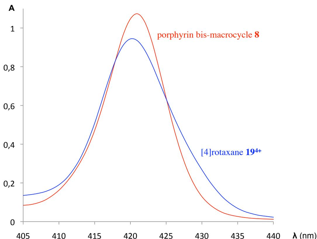
**Figure III.12.** UV-visible absorption spectra (Soret band) of [4]rotaxane **19<sup>4+</sup>** and its precursor, porphyrinic bis-macrocycle **8** in CH<sub>2</sub>Cl<sub>2</sub> with [porphyrin] = 1.9\*10<sup>-6</sup> M. The blue shift and broadening of the Soret band of the rotaxane is attributed to exciton coupling between the two central porphyrins.
