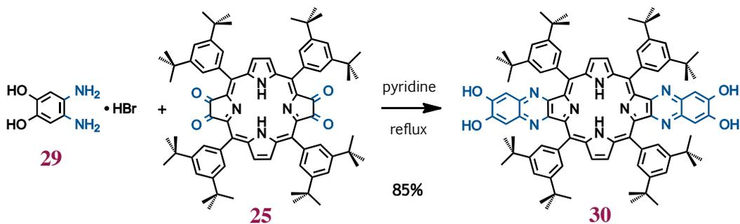
**Figure IV.9.** Synthesis of the linear bis(dihydroxyquinoxalino)-porphyrin **30**.
