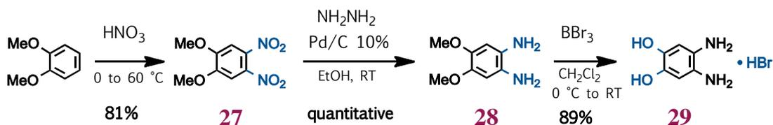
**Figure IV.8.** Synthesis of 4,5-diaminocatechol hydrobromide **29**.<sup>275</sup>
