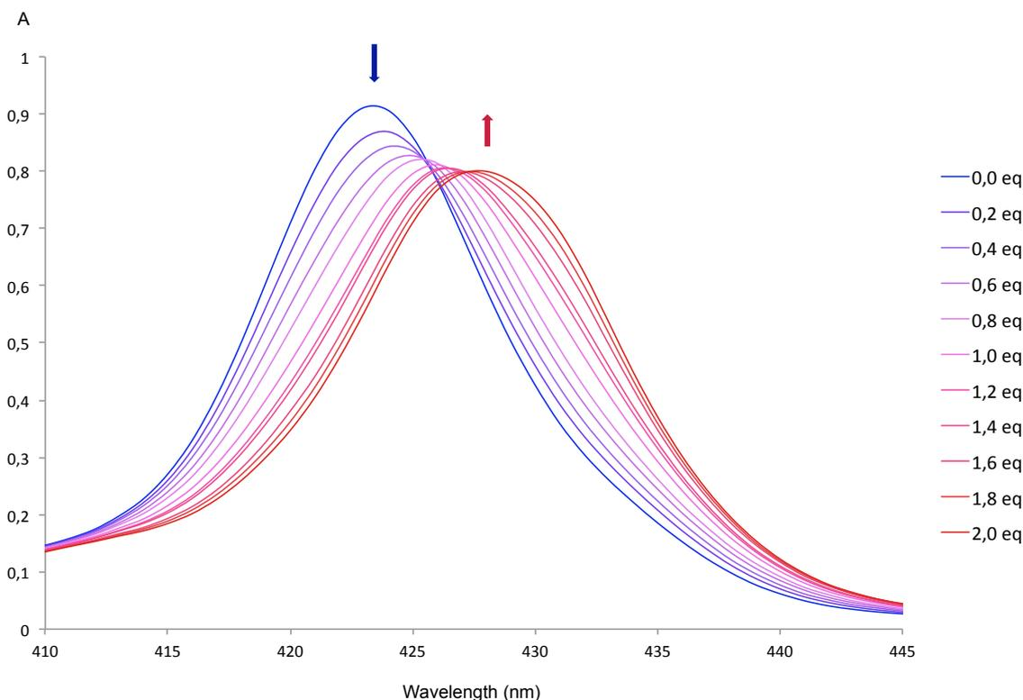
**Figure III.17.** UV-visible titration spectra in toluene (Soret band) of rotaxane **19**<sup>4+</sup> ( $0.92 \times 10^{-6}$  M) with DABCO guest **G1** ( $2.8 \times 10^{-5}$  M) from 0.0 to 2.0 equiv. Arrows show changes in the host spectrum with increasing guest concentration; a 6 nm red shift from 423 to 429 nm is observed.
