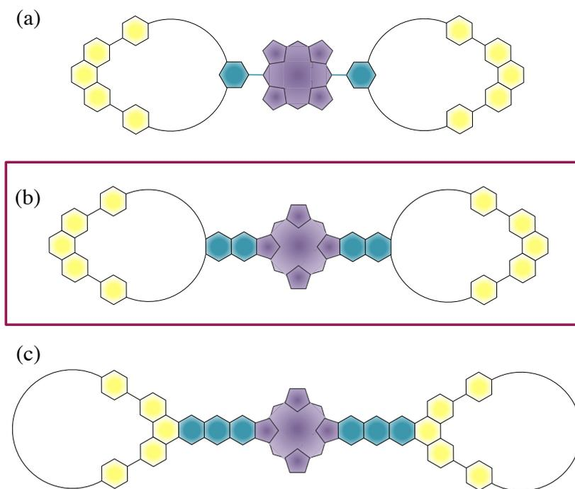
**Figure IV.1.** Schematic view of the structural differences between three porphyrinic bis-macrocycles: (a) compound **8** described in Chapters II and III of this thesis; (b) new target compound;<sup>196,197,217</sup> (c) compound used in previous studies.<sup>196,197,217</sup> The rigidity of the new system will be intermediate between the very flexible bis-macrocycle **8** and the very rigid bis-macrocycle studied by former members of the Sauvage group.
