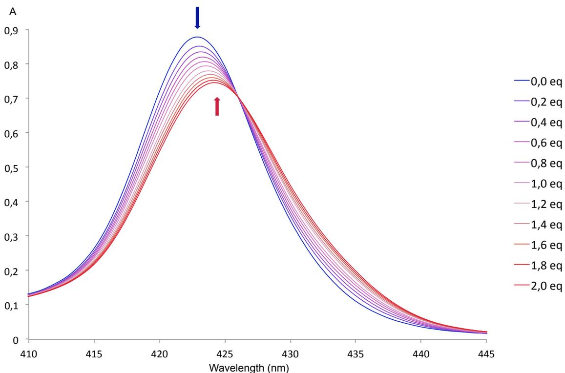
**Figure III.21.** UV-visible titration spectra in toluene (Soret band) of rotaxane **19**<sup>4+</sup> ( $0.92 \times 10^{-6}$  M) with guest **G4** ( $2.8 \times 10^{-5}$  M) from 0.0 to 2.0 equiv. Arrows show changes in the host spectrum with increasing guest concentration; a 1 nm red shift from 423 to 424 nm is observed.
