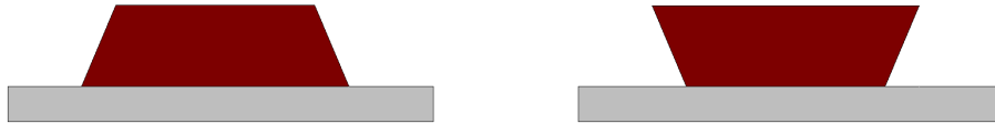
Figure 4.7: Schematic cross-sectional view of positive (left) and negative (right) photoresists after their UV insulation and development. Note the overhang of the negative PR.
