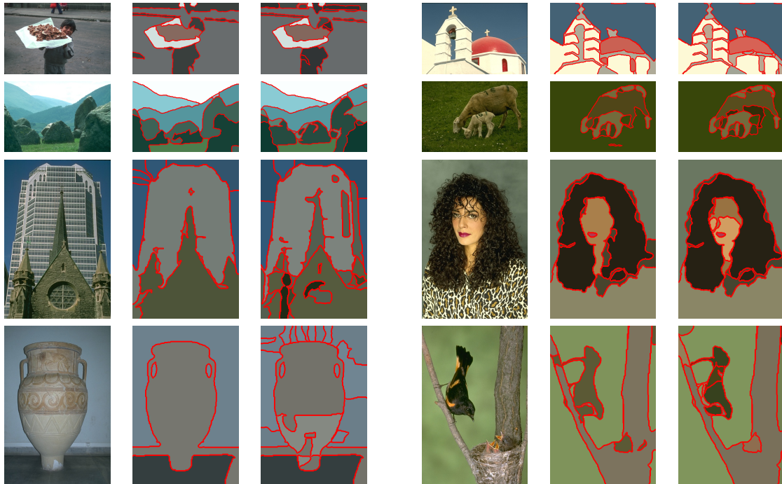
FIGURE A.13 – Segmentation results on images from the Berkeley database, using a superpixels initialization. All images were initialized at K = 15 classes. From left to right, each column shows the original image, the segmentation for \epsilon = 3 and the segmentation for \epsilon = 10 .
