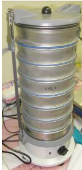
Figure 6.7 Debris mechanical sieve
