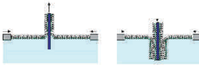
Figure 2.9: Scheme of the Langmuir-Blodgett deposition technique. The glass slide is taken out of the water subphase, inducing the deposition of a first lipid monolayer. By returning to the water phase and crossing a second time the interface, a second monolayer is deposited, leading to a supported bilayer.
