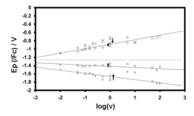
**A 12:** Plot of  $E_p$  vs. Log(v) for  $H_4L$ : 1 mM (square) and 5 mM (cross). Arrows show measurements performed with both Pt electrode and Pt microelectrode at 1 V.s<sup>-1</sup> to indicate that resistance effect is not the only limitation.
