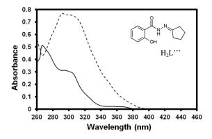
**A5:** Absorbance spectra of  $H_2L'(dotted line)$  and  $H_2L'''(thin line)$ , both at 5 10<sup>-5</sup> M
