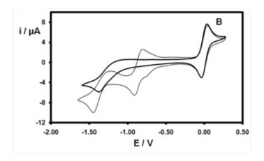
**A 10:** A)  $H_4L$  (thick line) and  $H_2L'$  (thin line) 1 mM,  $v = 0.02 \text{ V.s}^{-1}$ . B)  $H_4L$  1 mM (thick line) and  $H_4L$  1 mM with HCl 1 mM (thin line),  $v = 0.1 \text{ V.s}^{-1}$ . Pt working electrode,  $TBAPF_6 = 150 \text{ mM}$ , the potential of ferrocene is arbitrary fixed to 0 V.
