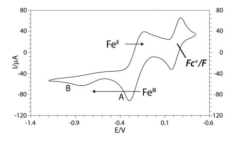
**Figure 12**: Cyclic voltammogram of 2 FeCl<sub>3</sub> and H<sub>4</sub>L 10 mM in DMF (TBA(PF<sub>6</sub>) = 0.15 M). Working electrode glassy carbon;  $v = 0.1 \text{ V s}^{-1}$ .
