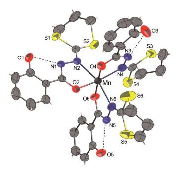
**Figure 2**: ORTEP view of the complex  $2 \cdot \text{CH}_2\text{Cl}_2$  with partial labelling scheme. The ellipsoids enclose 50% of the electronic density. The solvent  $\text{CH}_2\text{Cl}_2$  was omitted for clarity. Selected distances (Å) and angles (°): Mn–N2 2.294(3), Mn–N4 2.088(4), Mn–N6 2.259(3), Mn–O2 1.922(3), Mn–O4 1.892(3), Mn–O6 1.894(3); O4–Mn–O6 177.3(2), O2–Mn–N4 167.3(1), N2–Mn–N6 161.5(1).
