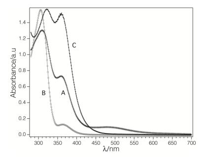
**Figure 14**: Absorption spectra of A) Fe<sub>2</sub><sup>III</sup>L, B) Fe<sup>II</sup>/H<sub>4</sub>L obtained after light exposure of Fe<sub>2</sub><sup>III</sup>L, and C) FeCl<sub>3</sub>. All solutions are about 1 mM in DMF.
