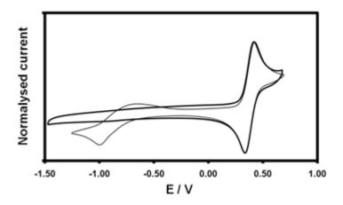
**A 7:** Cyclic voltammograms of  $H_4L$  (5 mM) recorded with carbon (thick line) and platinum (thin line) electrodes. DMF,  $TBAPF_6 = 150$  mM, v = 0.1 V.s<sup>-1</sup>.
