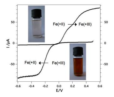
**Figure 11:** Quasi-steady-state current-potential curves measured for the virgin  $Fe^{III}$  and the photoreduced  $Fe^{II}$  species at 1.25 mM in DMF (nBu<sub>4</sub>NPF<sub>6</sub> 0.15 M). Working electrode: glassy carbon.  $v = 2 \text{ mV.s}^{-1}$  and rotation rate is 1000 rpm.
