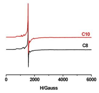
**Figure A7**: EPR spectra of  $\bf C8$  and  $\bf C10$  complexes recorded at 20K in frozen DMF solution at  $10^{-2}$  M.
