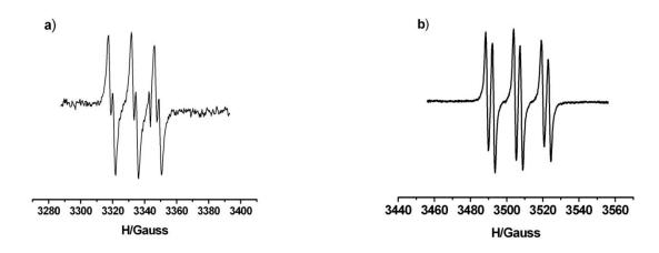
**Figure 11:** EPR spectrum showing the spin adduct obtained after irradiation in the visible at room temperature in the presence of  $3\times10^{-2}$  mol/L of PBN with  $10^{-2}$  M of a mixture of a) one equivalent of FeBr<sub>3</sub>, two equivalent of H<sub>2</sub>L b) one equivalent of FeCl<sub>3</sub>, two equivalent of H<sub>2</sub>L.
