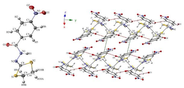
**Figure 14:** On the left ORTEP View for **HL**". On the right stacking view belon the lattice (X, 0, Z) (dashed Green line interaction between centre of the benzene ring (C1 - C6) and (C1-C6)"; dashed red line interaction between O1 and C5' via H5'; dashed black line interaction between N2 and N1" via H1")/ ' is the symmetry code x, -1+y, z; " is the symmetry code -x,-1/2+y, 1/2-z and "" is the symmetry code -x,-y,-z.
