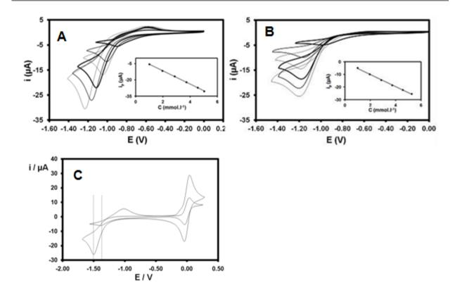
A 8: Cyclic voltammograms of A) H<sub>4</sub>L and B) H<sub>2</sub>L' for different concentrations: 1, 1.95, 2.85, 3.72, 4.54 and 5 mM. C) Cyclic voltammogram of H<sub>4</sub>L for 1 mM and 5 mM with ferrocene to calibrate the potentials. DMF, Pt working electrode, Pt pseudo reference electrode, TBAPF<sub>6</sub> = 150 mM, v = 0.1V.s-1, (insert: Ip vs. C)
