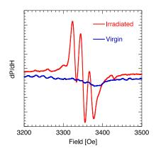
Fig A13: EPR spectra of the iron complex in DMF at 6 K: blue line before irradiation, red line after 3 hours of irradiation.
