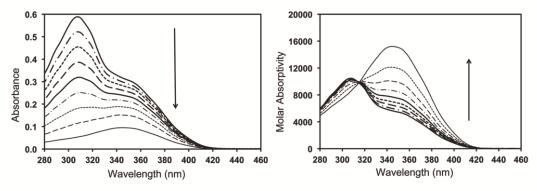
**Figure 8:** Absorption spectra and its relative molar absorptivity of H<sub>4</sub>L for different concentrations in DMF: 5.6, 5.0, 4.4, 3.7, 3.1, 2.5, 1.9, 1.3 10<sup>-5</sup> M and 6.3 10<sup>-6</sup> M (The arrow indicates the sense of the absorbance changes with decrease of the concentration)
