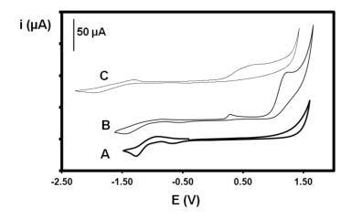
**A 6:** Cyclic voltammograms of A)  $H_4L$ , B)  $H_2L$  and C)  $H_4L$  : C = 5mM, Pt working electrode, Pt pseudo reference electrode,  $TBAPF_6 = 150 \text{ mM}$ ,  $v = 0.1 \text{ V.s}^{-1}$
