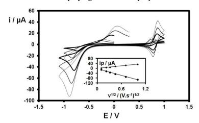
**A 9:** Cyclic voltammograms of  $H_4L$  (5 mM) for different scan rates :0.01, 0.05, 0.1, 0.2, 0.5 and 1 V.s<sup>-1</sup>. Pt working electrode,  $TBAPF_6 = 150$  mM (Insert: Ip vs.  $v^{1/2}$ )
