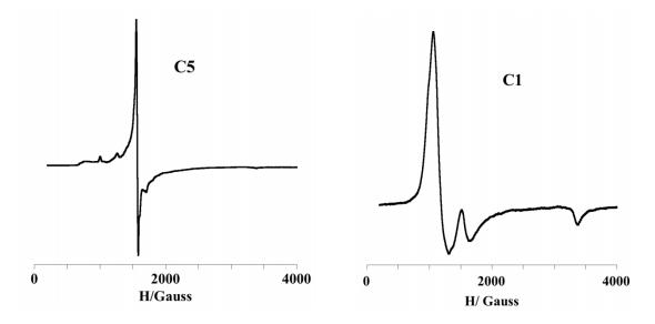
**Figure 12**: EPR spectra recorded in frozen DMF solution at low temperature (6K). right for C1(10<sup>-2</sup> M) and left for C5 (10<sup>-2</sup> M)
