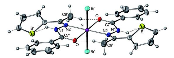
**Figure 2**: ORTEP view of complex **1** with a partial labelling scheme. Hydrogen bonds (intra molecular) are represented in dashed lines. The ellipsoids enclose 50% of the electronic density. Symmetry code for ' = -x, -y, -z. Selected distances (Å): Br–Ni 2.5502(5), Ni–O 2.036(4), Ni–N2 2.120(5), O–C7 1.233(6), N1–C7 1.352(7), N1–N2 1.404(7)
