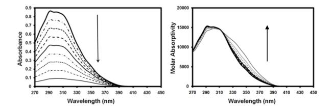
**A1:** Absorption spectra (left) and molar absorptivity (right) of H<sub>2</sub>L' for different concentrations: 5.6 10<sup>-5</sup> M, 5.0 10<sup>-5</sup> M, 4.4 10<sup>-5</sup> M, 3.7 10<sup>-5</sup> M, 3.1 10<sup>-5</sup> M, 2.5 10<sup>-5</sup> M, 1.9 10<sup>-5</sup> M, 1.3 10<sup>-5</sup> M and 6.3 10<sup>-6</sup> M (The arrow indicates the sense of the absorbance changes with decrease of the concentration)
