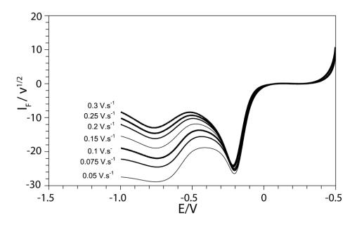
**Figure 13**: Half cyclic voltammograms of  $2\text{FeCl}_3$  and  $H_4\text{L}\ 1$  mM at different scan rates in DMF (TBA(PF<sub>6</sub>) = 0.15 M). Working electrode: glassy carbon. I<sub>F</sub> is the Faradic current obtained after subtracting the capacitive current.
