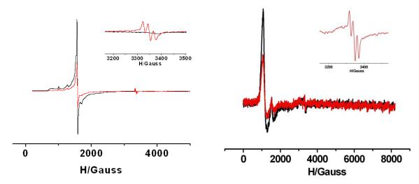
**Figure 13**: On the left EPR spectra of Fe(**HL**)<sub>2</sub> (DMF)(Cl) 10<sup>-2</sup> M in DMF at 80 K: black line before irradiation, red line after 3 hours of irradiation. On the left EPR spectra of Fe(**HL**)<sub>2</sub>(DMF)(Br) 10<sup>-3</sup> M in DMF at 120K: black line before irradiation, red line after 3 hours of irradiation.
