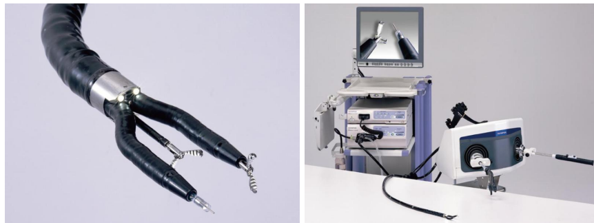
Fig. 2.25. Olympus EndoSamurai with its control console (reprinted from [165]).
