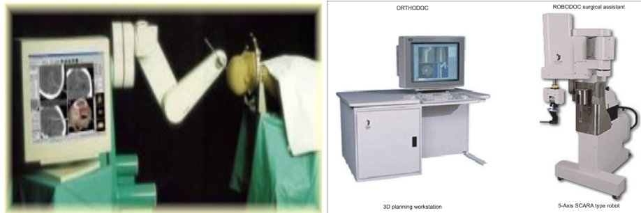
Fig. 3.1. Left: First version of the Neuromate robot (reproduction from http://www.emsmedical.net ). Right: Robodoc (reprinted from [178]).
