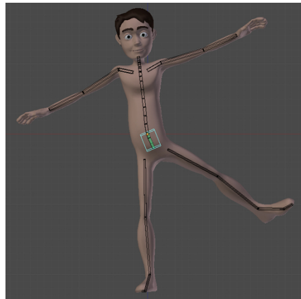
Fig. 5.23. An example of character mesh modified by an armature in Blender (reprinted from [191]).
