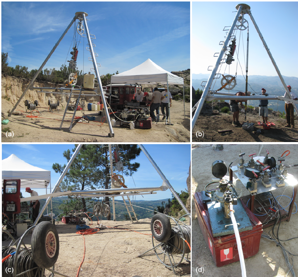
Figure 2.9: Hydraulic tests performed at the Paradela II site: (a) general view of the testing scheme, (b) downward movement of the upper packer, (c) downward movement of the system with the coiled tubing and (d) hydraulic pump.
