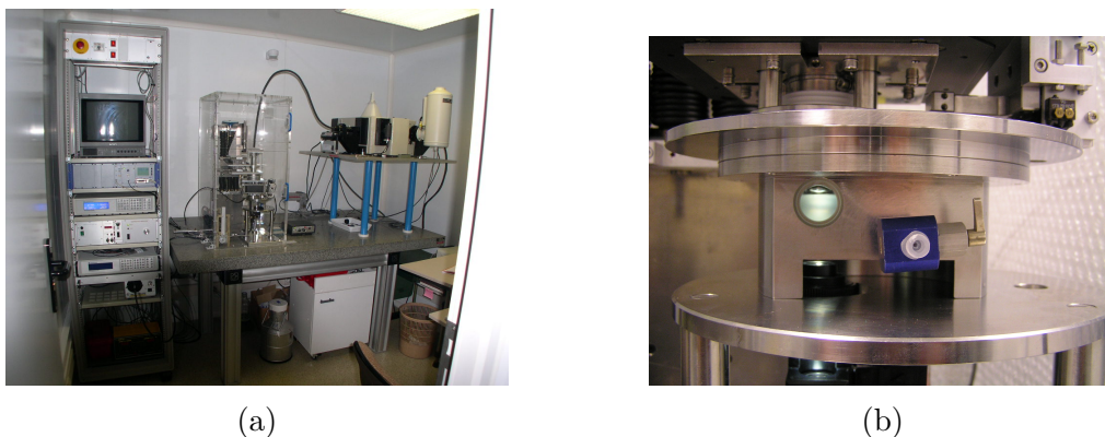
Figure 2.5: Figure (a): setup of the SFA, on the left the electronics, in the middle the SFA chamber in the plexiglas cabinet, on the right the spectrometer. Figure (b): SFA chamber filled with a lamellar mesophase, through the window, the surfaces are almost not visible due to the non translucent sample.
